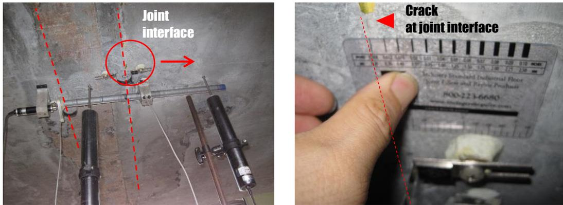
(a) cracks on the bottom surface
