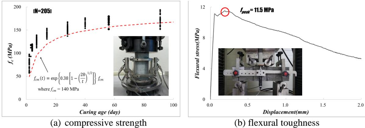
(a) compressive strength (b) flexural toughness
