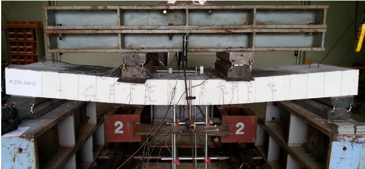
Fig. 5 Failure of specimens upon completion (P-250-160-U)
