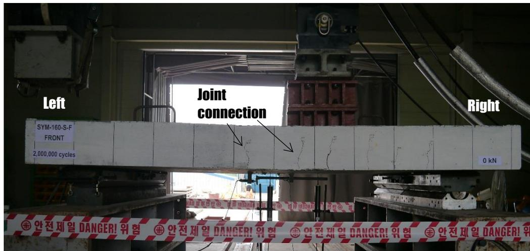
Fig. 11. Distribution of the crack over the length upon the completion of the fatigue test (SYM-160-S)
