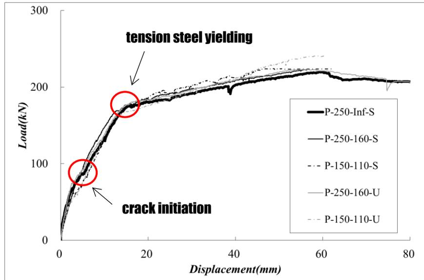
Fig. 4 Load and displacement relationship (Note: 1kip = 4.45 kN, 1in. = 25.4 mm)
