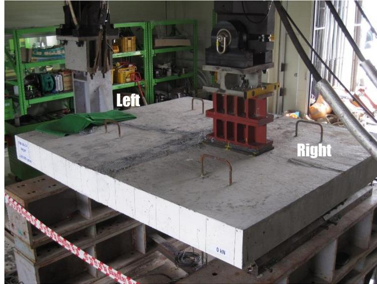
Fig. 9 Overview of fatigue test set-up
