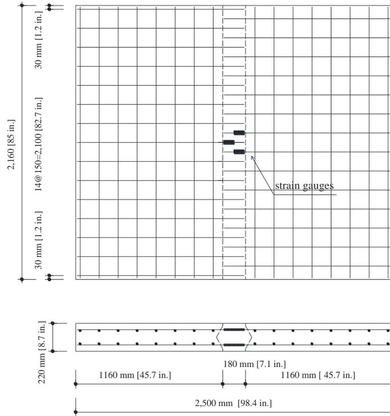
Fig. 7 Geometry of the precast deck specimens (Note: 1 in. = 25.4 mm)
