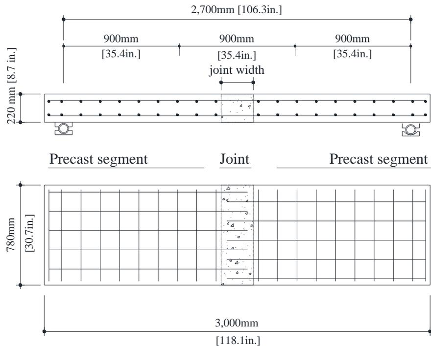
Fig. 3 Geometry of the precast beam specimens (Note: 1 in. = 25.4 mm)
