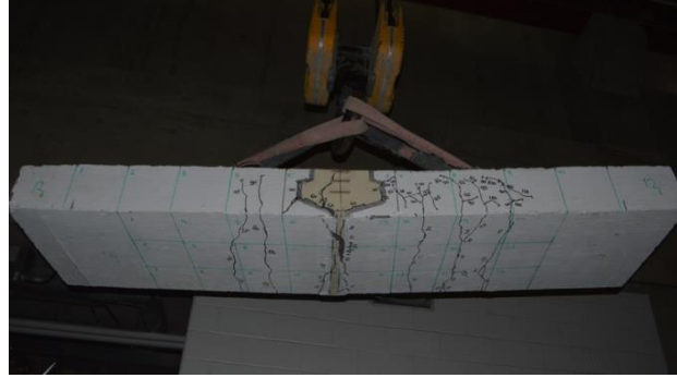
d) Flexural crack at bottom of the joint
