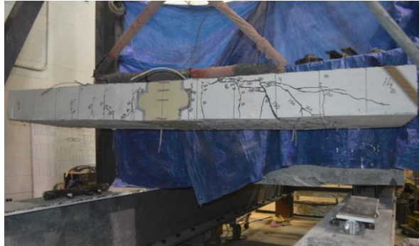
b) Crack pattern at the joint region
