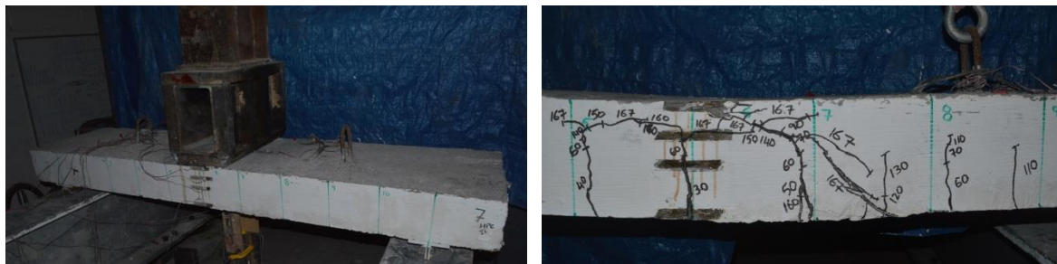
Fig. 7 Test setup and crack pattern at failure of slab S1
