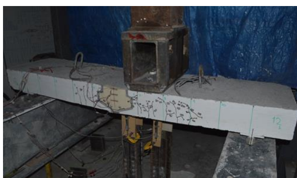
b) Crack pattern at the joint region
