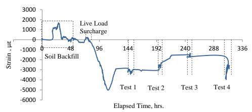
Fig. 22. Strain vs. elapsed time in steel at top reinforcement of the base 1 ft. from middle counterfort
