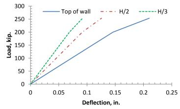
Fig. 7 Load vs. deflection plots using ANSYS Package
