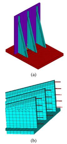
Fig. 6 Finite element model of (a) TPCCRW and (b) anchors extending from counterforts
