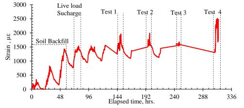
Fig. 19 Strain variation curve at the times of testing for Anchor 1 in Left Counterfort
