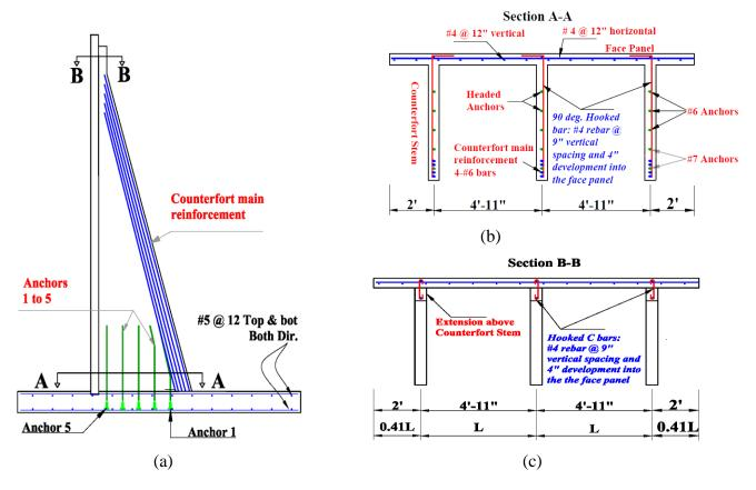
Fig. 5 Side elevation of TPCCRW with section A-A and section B-B
