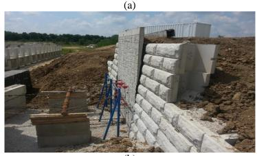
(b) Fig. 15 Experimental test setup showing hydraulic cylinders and steel rod
