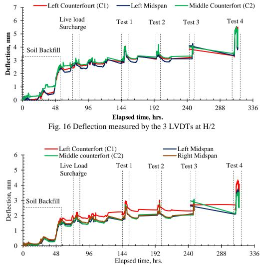
Fig. 17 Deflection measured by the 3 LVDTs at H/3
