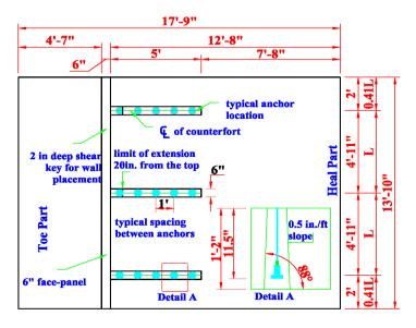
**Top View** Fig. 4. TPCCRW elevations and dimensions
