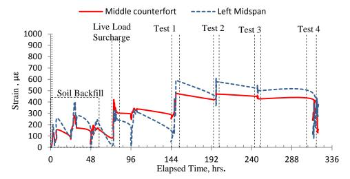
Fig. 20 Strain vs. time readings for face-panel steel reinforcement located at H/3 at the middle counterfort and left midspan
