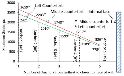
Fig. 18 Maximum strains in headed anchors at the middle and Left counterforts
