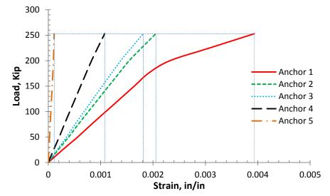
Fig. 9 Applied load vs. strain at each anchor in the middle counterfort from ANSYS
