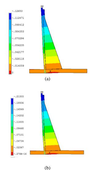
Fig. 8 Deflection contour at (a) service load (152 kip) (b) ultimate load (253.5kip) (ANSYS Package)
