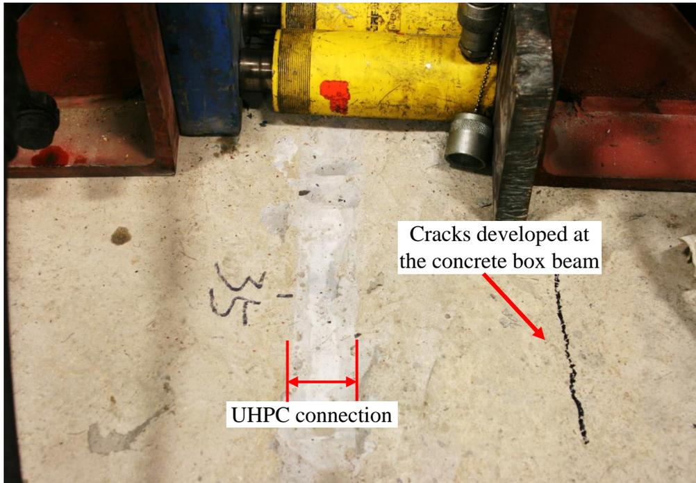
Fig.24 Mechanically Crack the Connection. Partial-Depth UHPC Connection.
