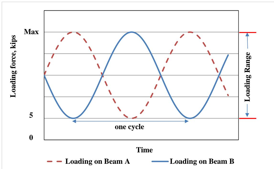
**Fig.7** Loading Protocol for Simply Supported Beams.
