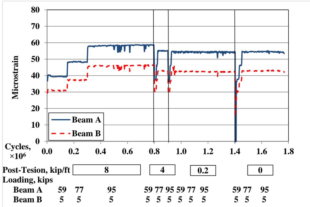
**Fig.20** Tensile Strain at Mid Span. Uncracked Partial-Depth Convention Grout, Restrained Deflection (Clamp Down Ends and Extra Supports Underneath Beam B)
