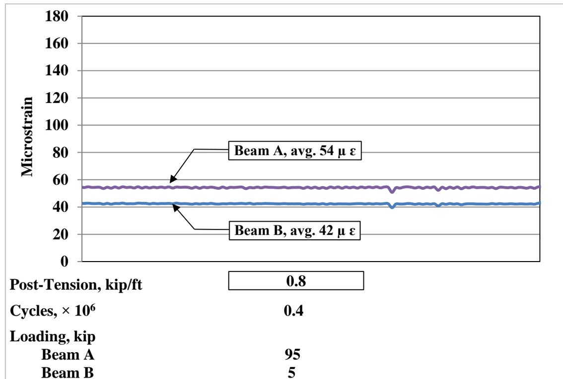
**Fig.16** Tensile Strain at the Mid-Span. Partial-Depth Conventional Grout, Restrained Deflection (Clamp Down Beam Ends and Extra Supports Underneath Beam B).
