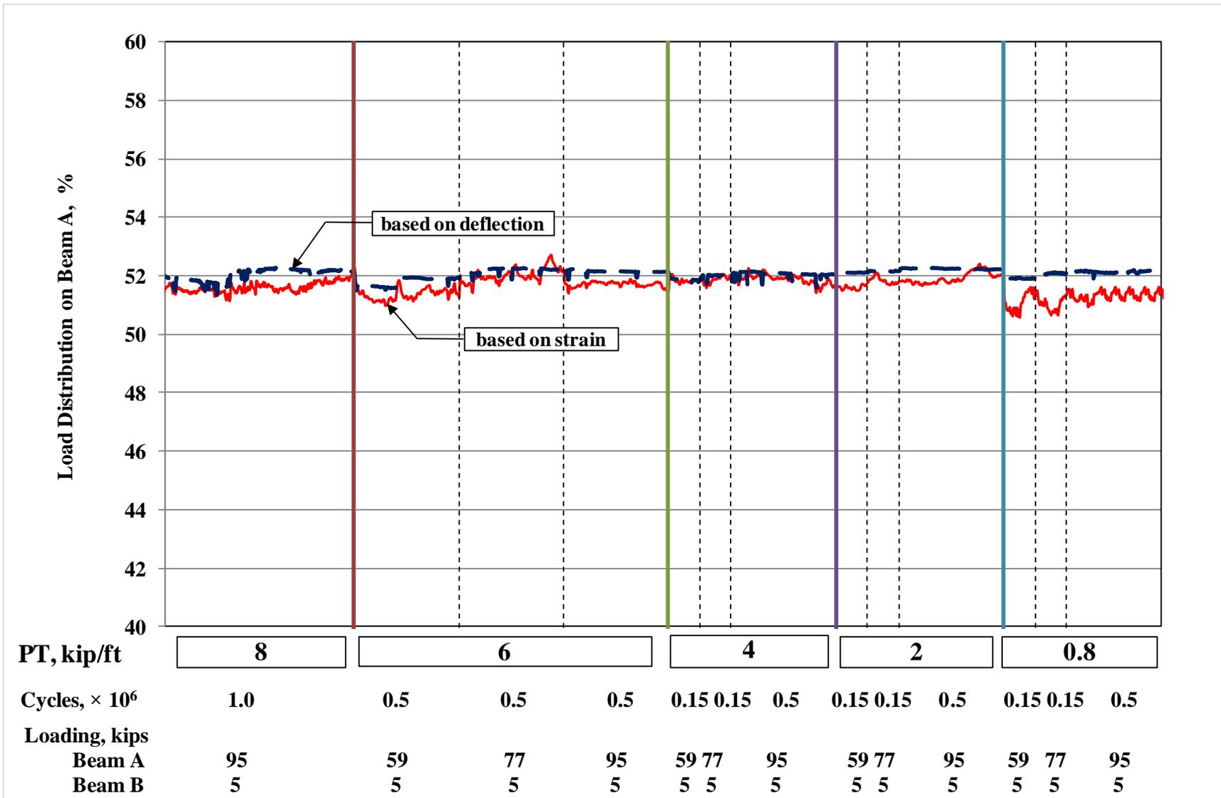
**Fig.18** Load Distribution at Different Loading Range and Transverse Post-Tension (PT) Level. Partial-Depth Conventional Grout, Simply Supported.
