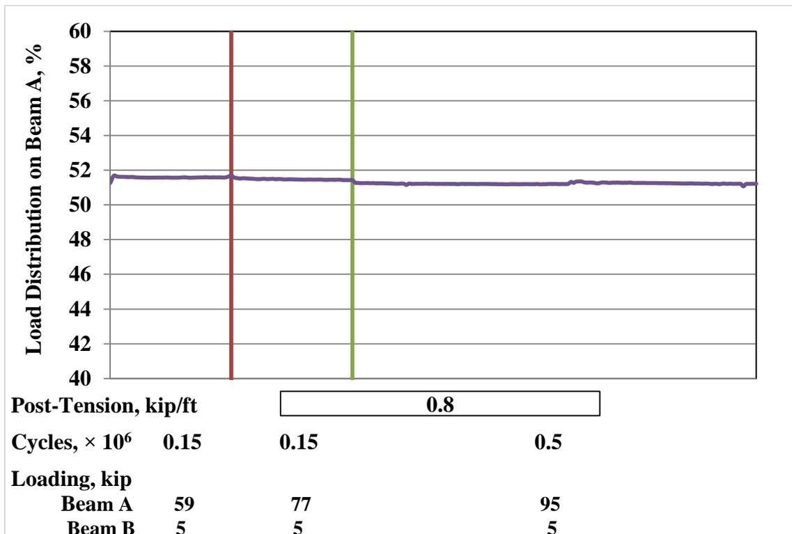
Fig.25 Load Distribution based on Tensile Strain. Partial-Depth Conventional Grout.
