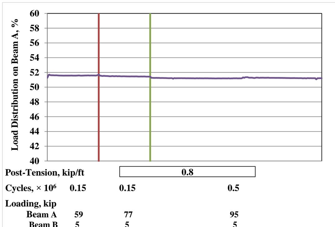
**Fig.13** Load Distribution based on Tensile Strain. Partial-Depth Conventional Grout, Clamp Down Beam Ends (No Extra Supports Underneath the Beam).
