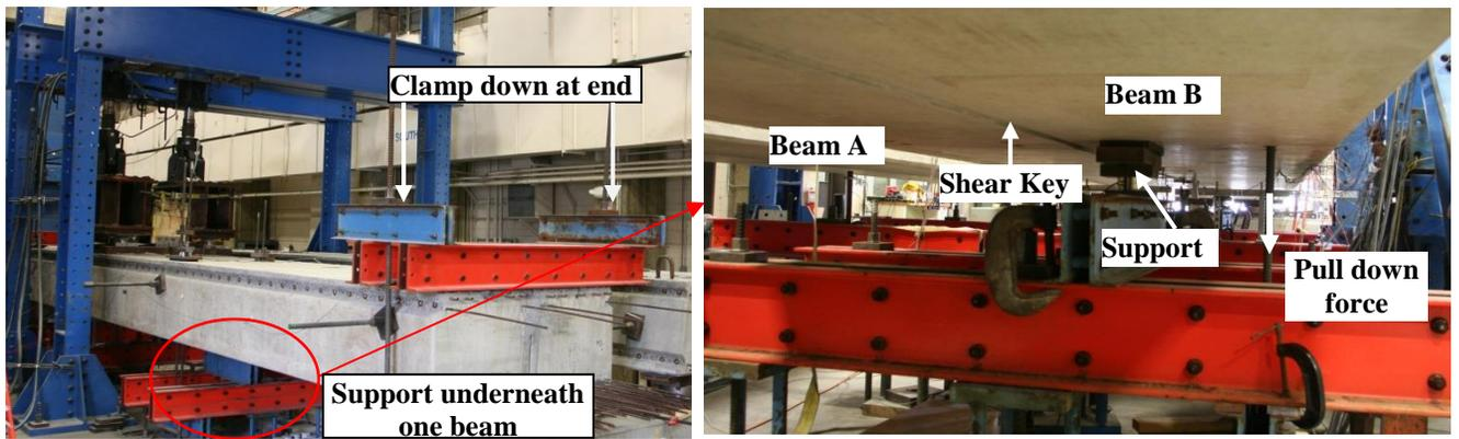
**Fig.9** Pictures of Clamping the End and Providing Extra Support Underneath One Beam
