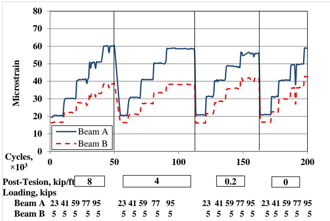
**Fig.22** Tensile Strain at Mid Span. Fully-Cracked Partial-Depth Conventional Grout, Restrained Deflection (Restrained End Rotation and Extra Supports Underneath Beam B)
