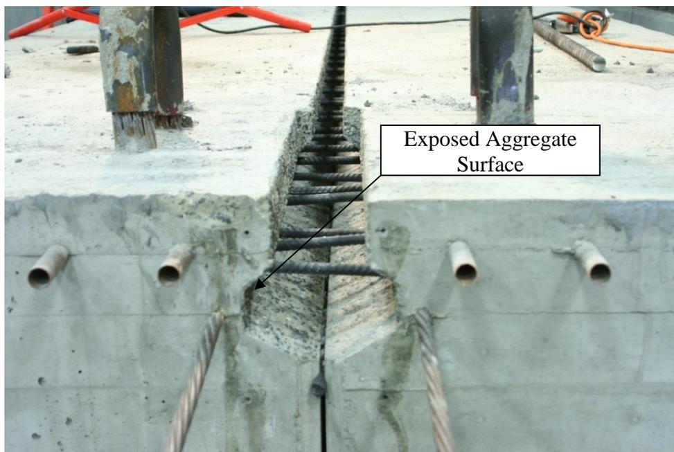
**Fig.5** Picture of UHPC Shear Key Design.
