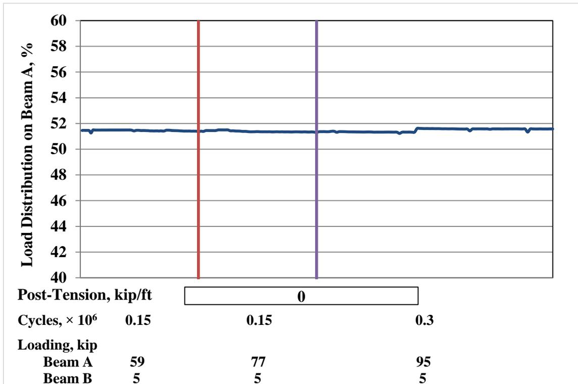
Fig.26 Load Distribution based on Tensile Strain. Partial-Depth UHPC Connection.
