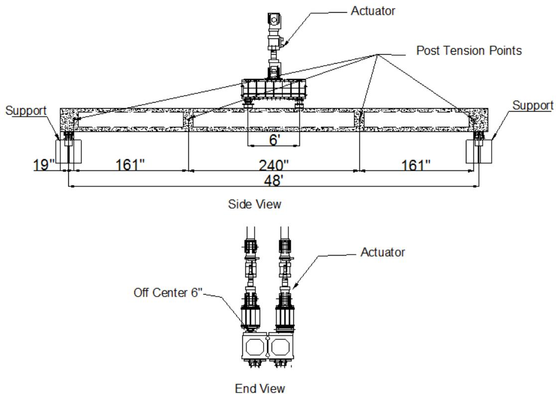
**Fig.6** Tests Setup for Simply Supported Configuration.
