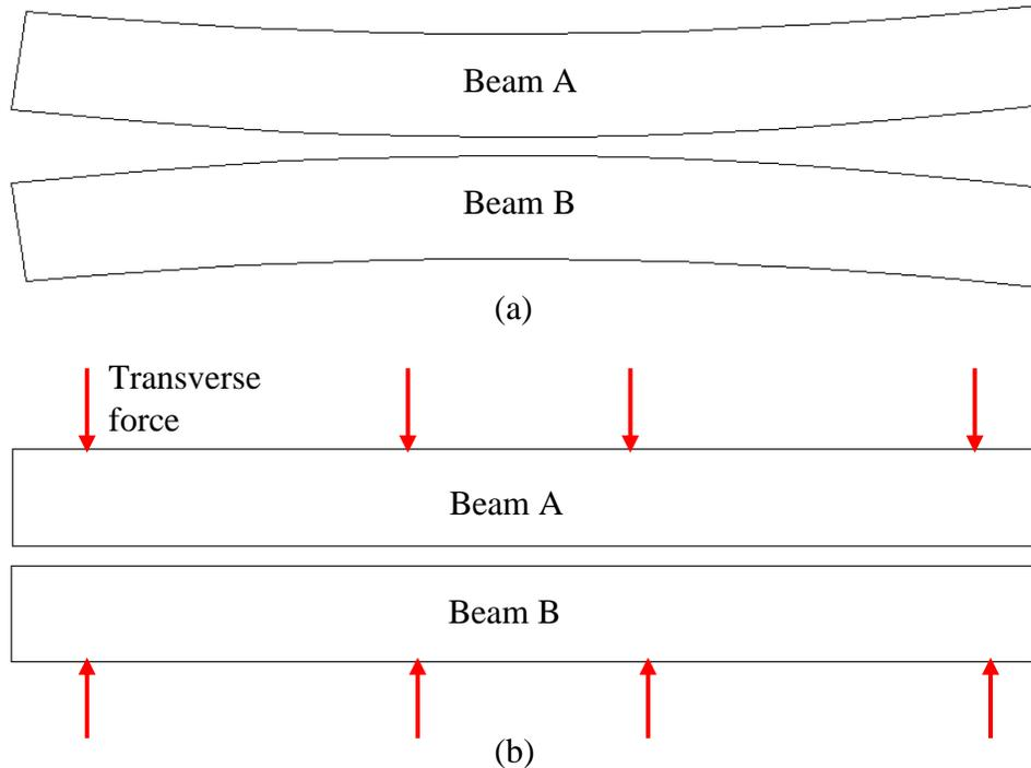
**Fig.23** (a) Curved Box Beams; and (b) Straightened Box Beams due Applied Transverse Force. (Exaggerated)
