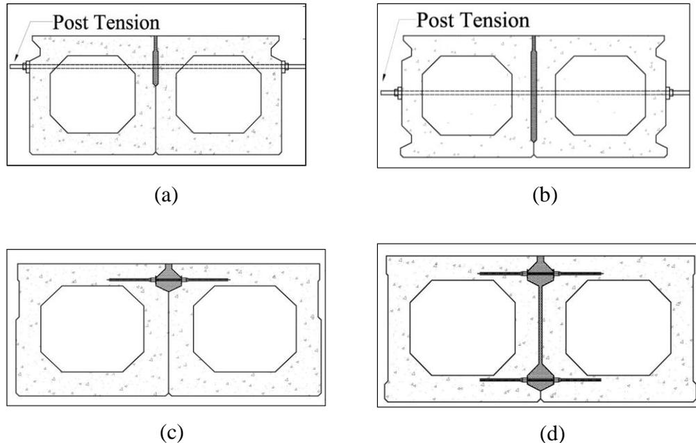
**Fig.1** Shear Key Connection: (a) Partial-Depth Conventional Grout; (b) Full-Depth Conventional Grout; (c) Partial-Depth UHPC; and (d) Full-Depth UHPC.
