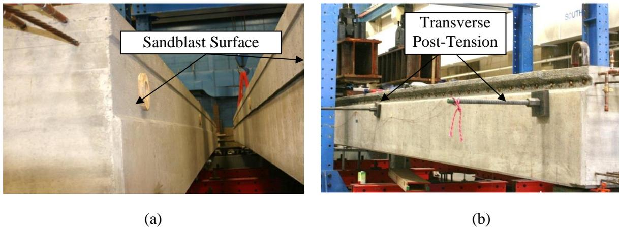
**Fig.4** Partial-Depth Conventional Grout Shear Key: (a) Sandblasted Surface; and (b) Transverse Post-Tension.
