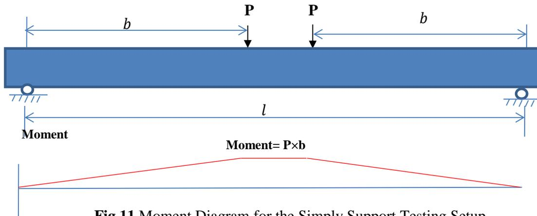
Fig.11 Moment Diagram for the Simply Support Testing Setup.
