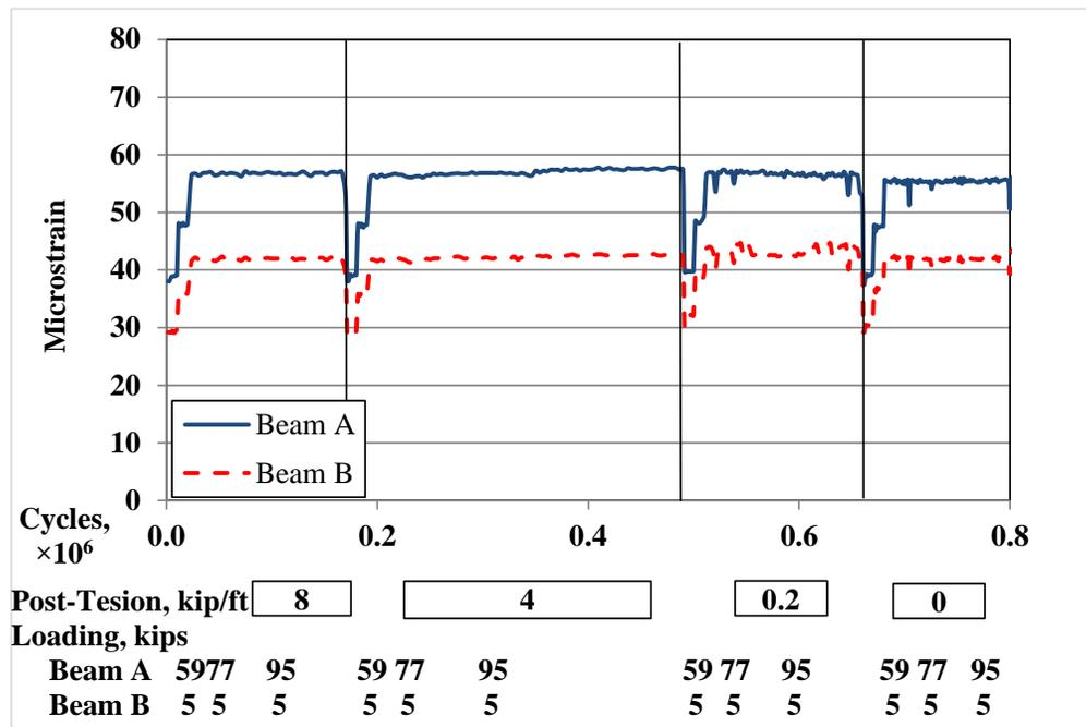
**Fig.21** Tensile Strain at Mid Span. Partially-Cracked Partial-Depth Convention Grout, Restrained Deflection (Clamp Down Ends and Extra Supports Underneath Beam B)
