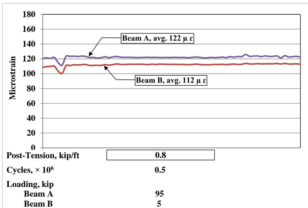
**Fig.15** Tensile Strain at the Mid-Span. Partial-Depth Conventional Grout, Clamp Down Beam Ends (No Extra Supports Underneath the Beam).
