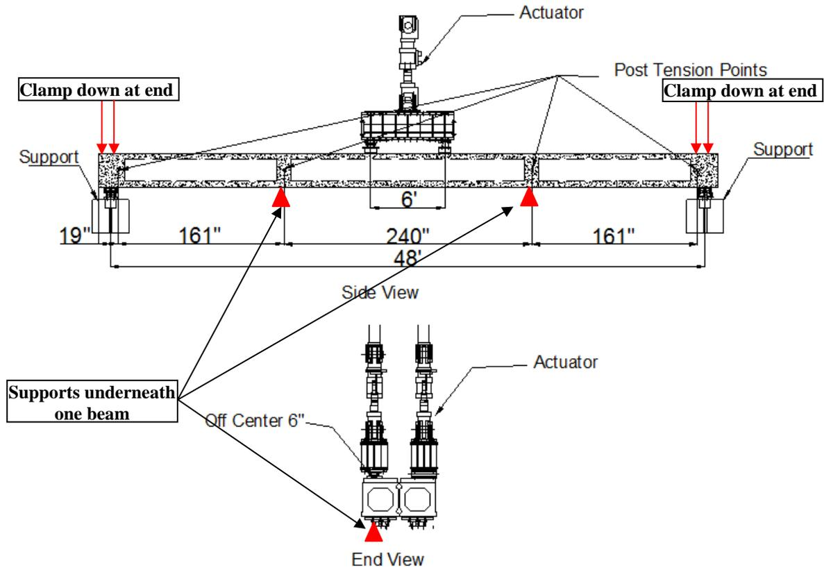
**Fig.8** Tests Setup for Restrained Deflection Configuration.
