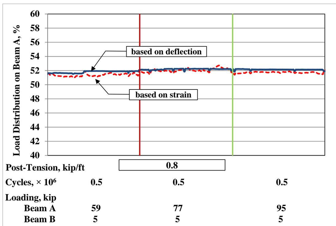
**Fig.12** Load Distribution based on Deflection and Tensile Strain. Partial-Depth Conventional Grout, Simply Supported.
