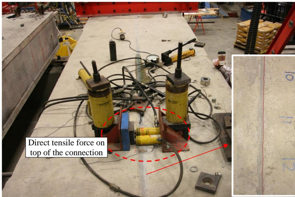
**Fig.19** Mechanically Crack the Connection. Partial-Depth Conventional Grout.
