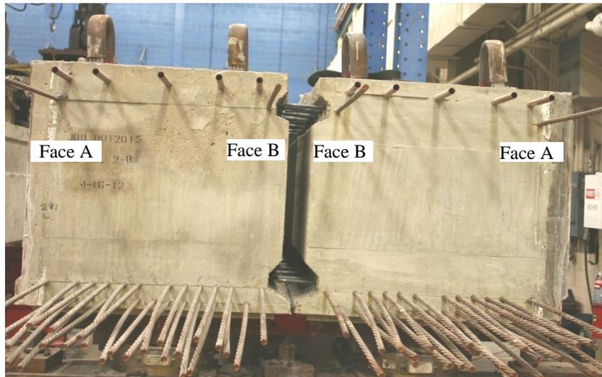
**Fig.3** Shear Key Design for Full-Depth Conventional Grout (Face A) and Full-Depth UHPC (Face B): (a) Dimension of the Box Beam Cross Section and Shear Key; and (b) Picture of the Box Beams.
