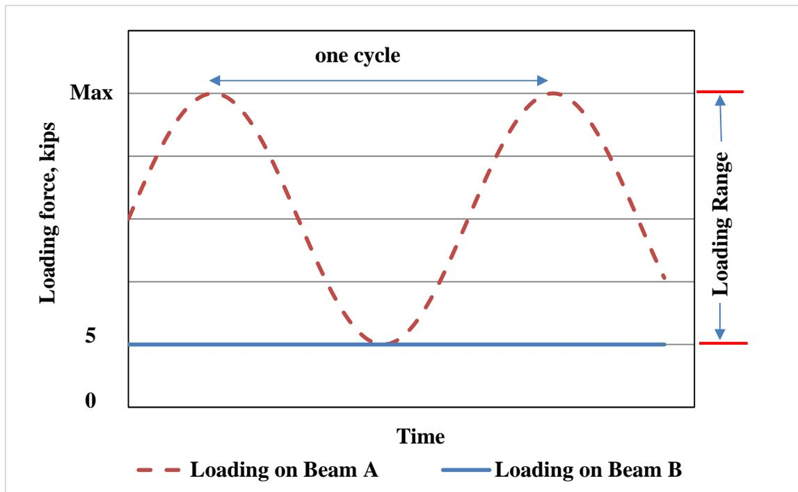
**Fig.10** Loading Protocol for Restrained Deflection Configuration.
