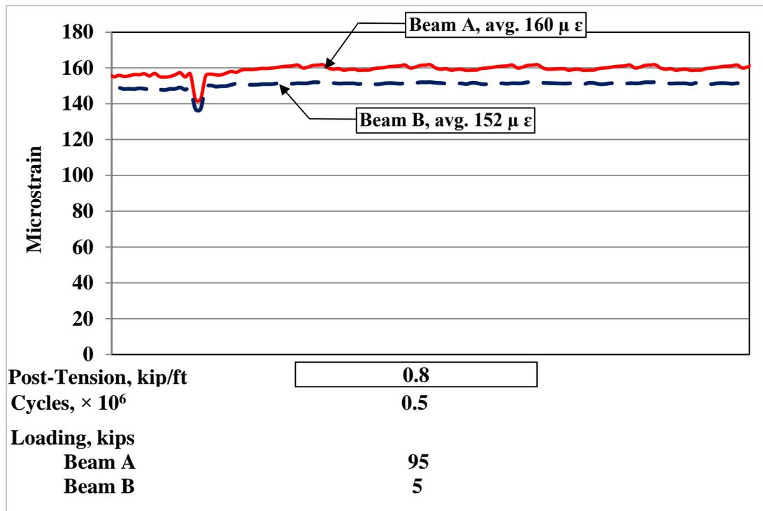
**Fig.14** Tensile Strain at the Mid-Span. Partial-Depth Conventional Grout, Simply Supported.
