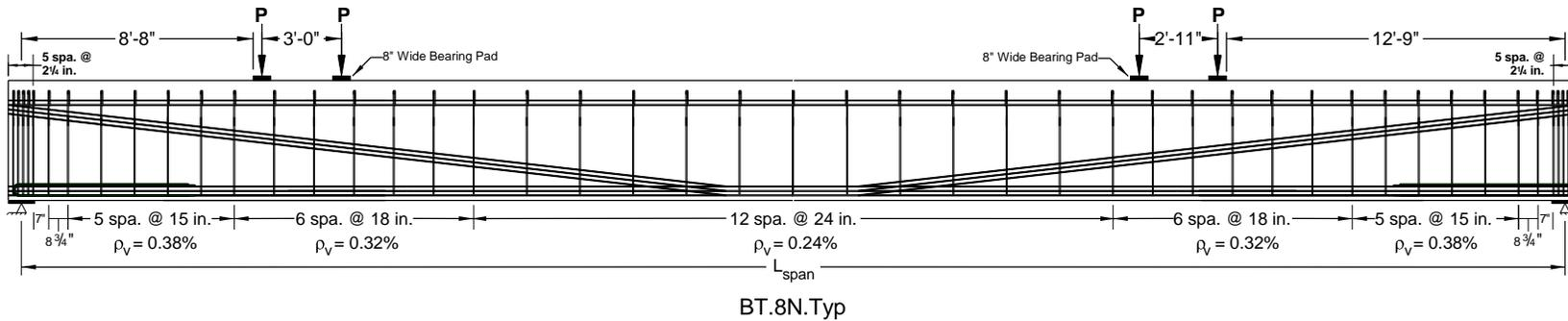
Figure 2. Elevation view of test girders showing stirrup spacing, harped prestress tendons, and concentrated load locations.
