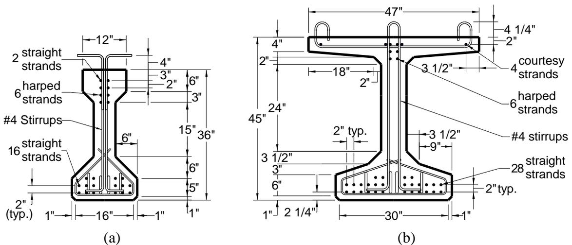
Figure 1. Cross-sectional geometry and reinforcement details for (a) AASHTO Type II girder and (b) PCBT-45 girder.
