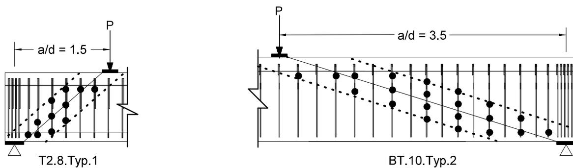
Figure 3. Locations of electrical resistance strain gages for two tests that are typical of other tests.
