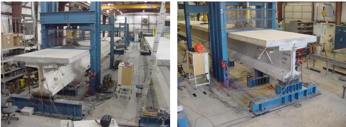
Figure 4. Photos of typical setups for load testing girders.
