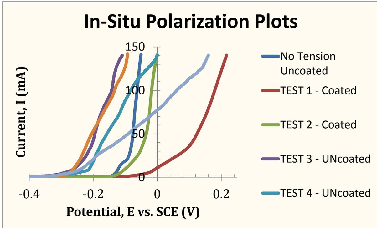
C wires while under stress; Tests #1-#6 are all on tensioned wires.
