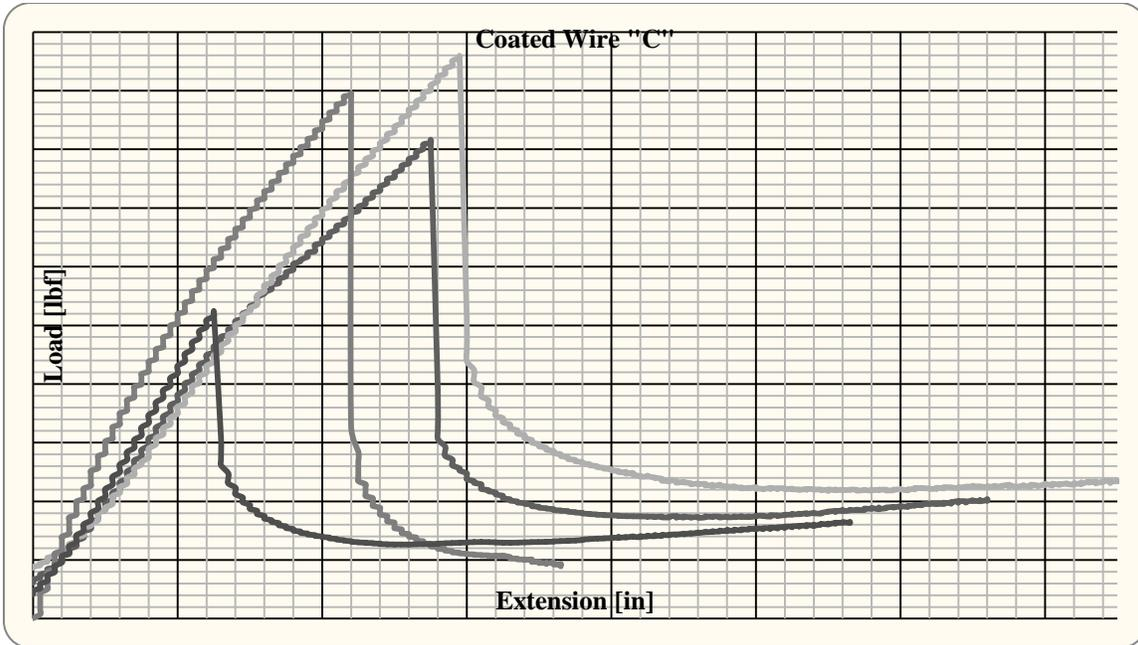
Figure 9. Load and slip or extension plot for coated wire C in pullout test.
