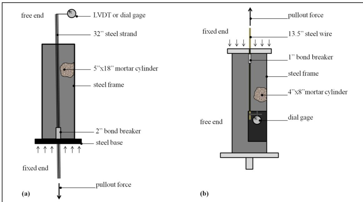
Figure 8. (a) NASP Bond Test setup and (b) Small-Scale Bond Test setup
