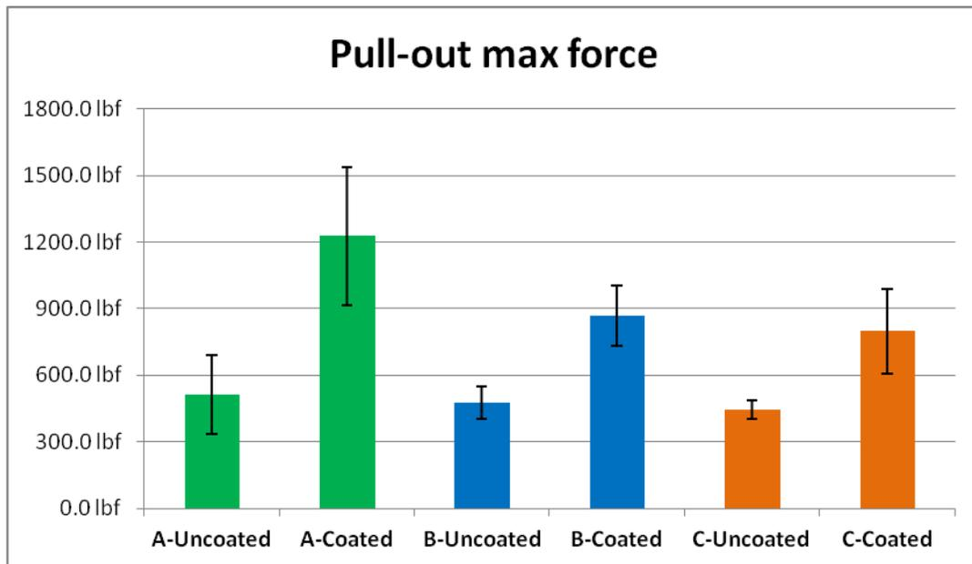
Figure 10. Comparison of wire pullout forces.
