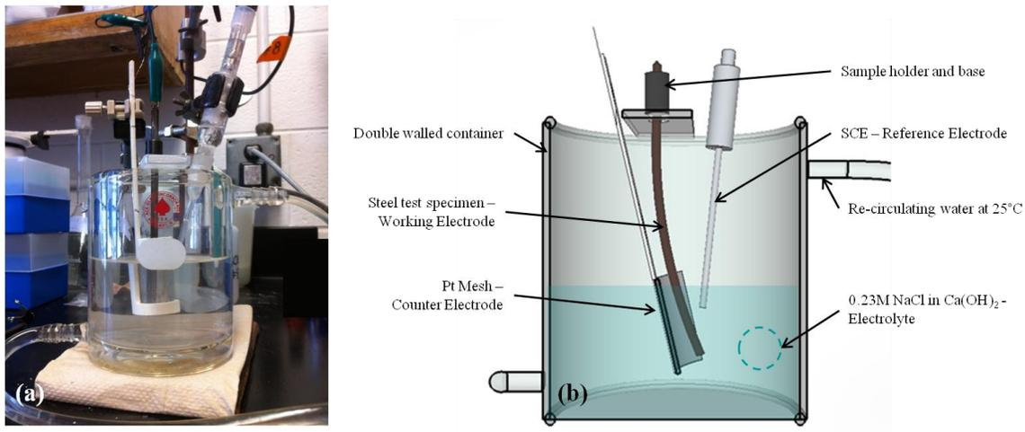
Figure 2. Three-Electrode Cell used for the polarization Experiments
