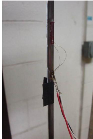
Figures 3, 4 & 5. (clockwise from top right): In-situ electrochemical test setup, strain gauge bonded to steel wire, and three-electrode potentiodynamic anodic polarization test surrounding tensioned wire.
