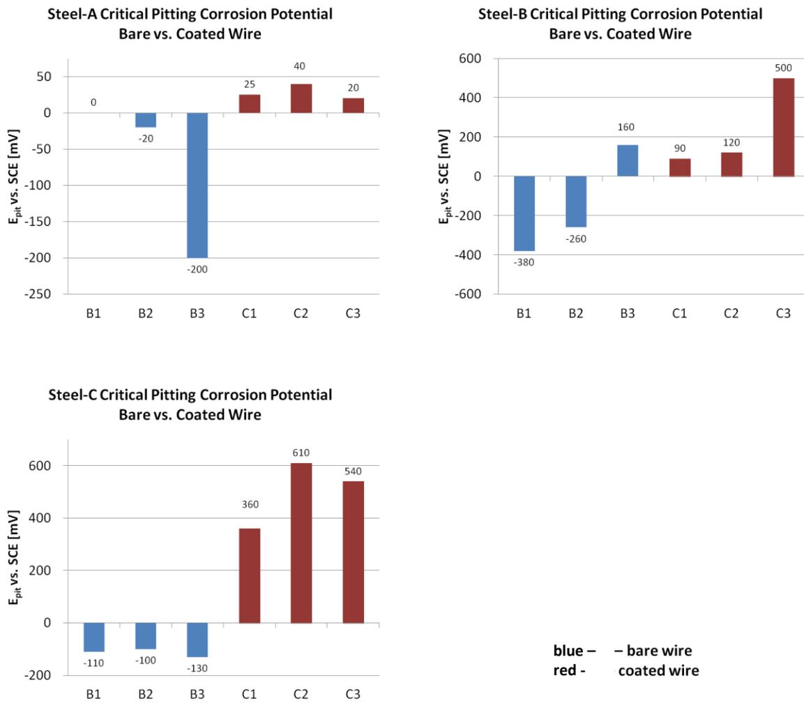
Figure 6. Test results showing pitting corrosion potential for test specimens.
