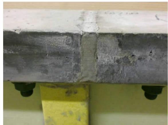
(a) Connected by mortar (Gap = 10 mm)
