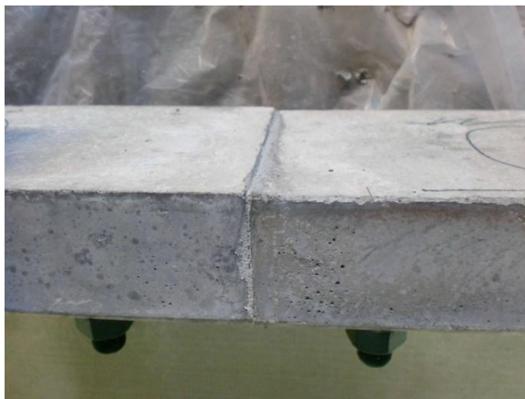
(a) Connected by epoxy bonding (Gap = 0)
