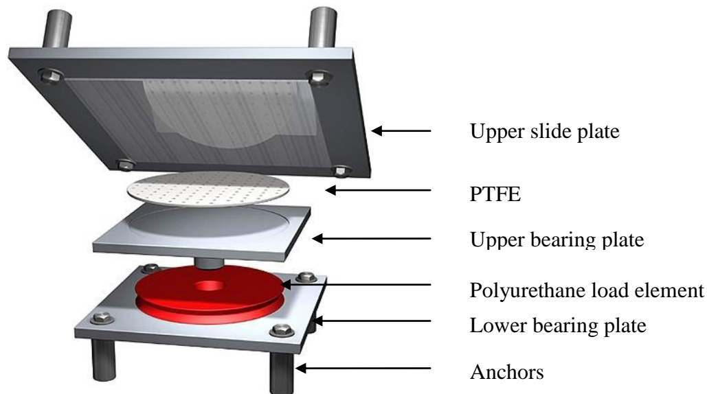
Fig. 3 Multidirectional disk bearing
