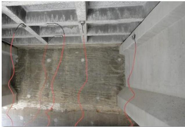
**Figure 5:** Transducers under Deck Adjacent to Abutment Face
