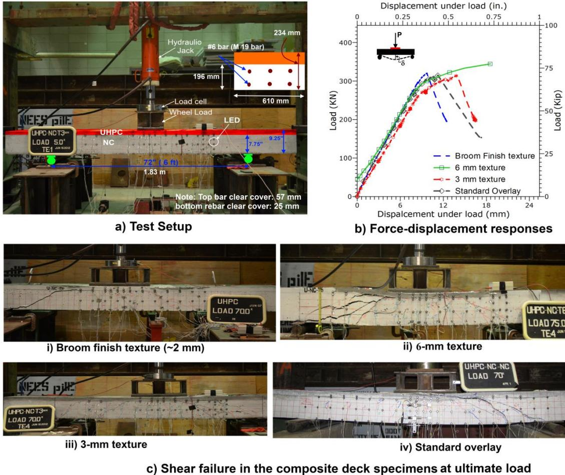
**Figure 3 Testing of UHPC-NC composite deck specimens**
