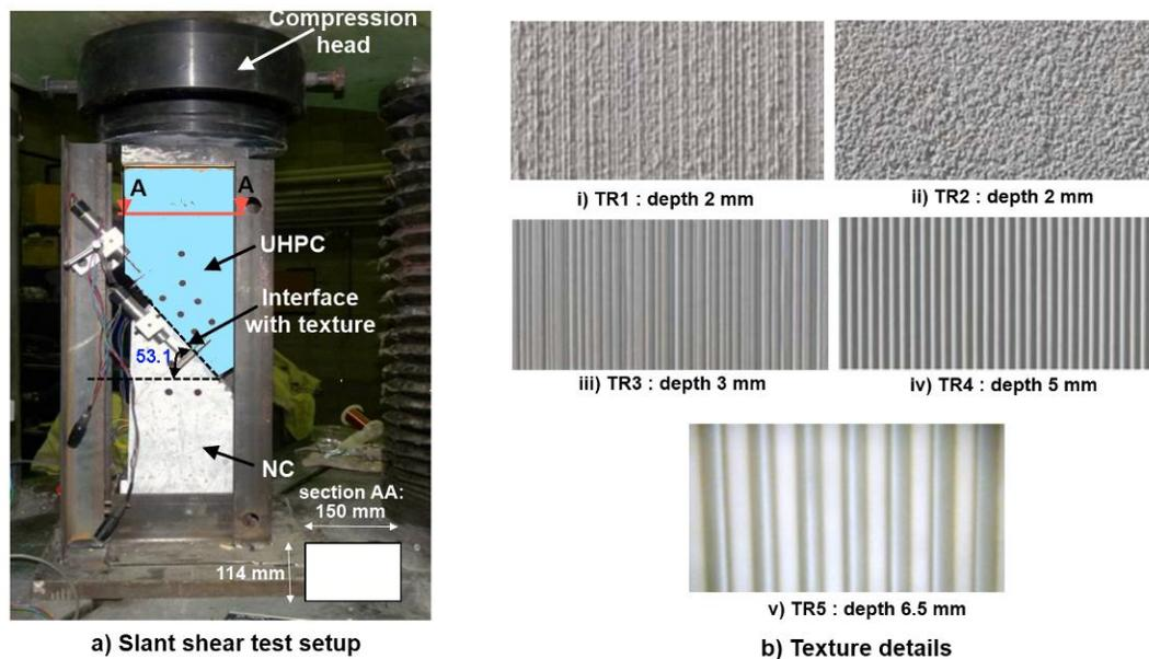
**Figure 1 Test setup and textures used for slant shear tests**
