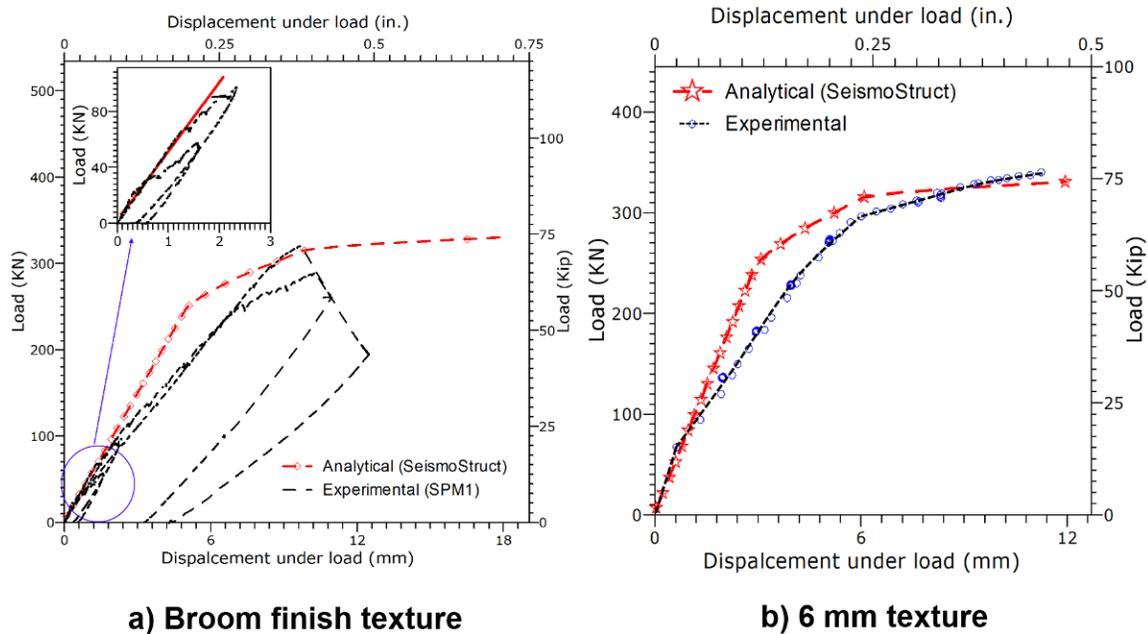
**Figure 4 Comparison of experimental and analytical force-displacement responses for two composite specimens**
