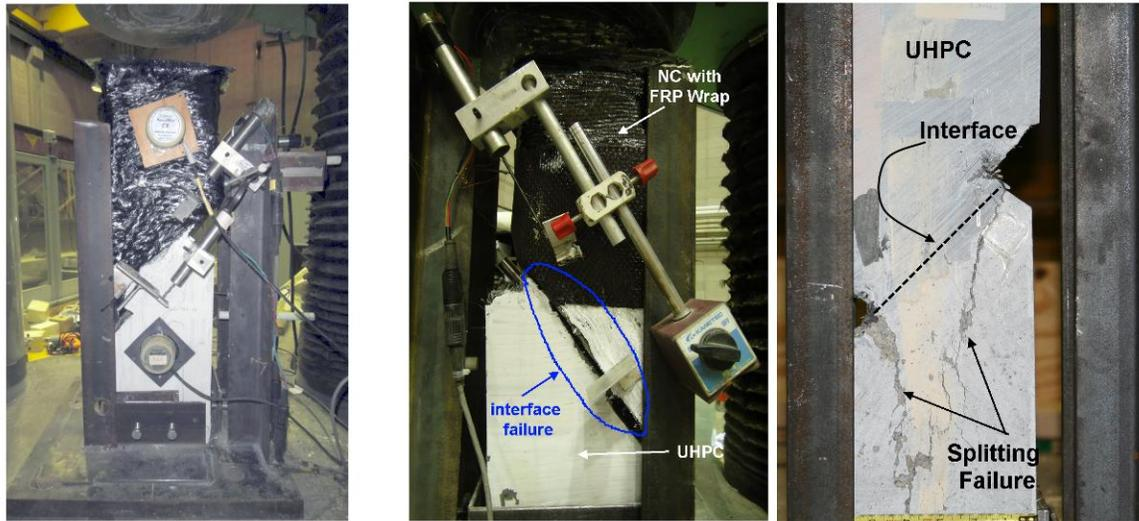
a) Normal concrete section strengthened with FRP
