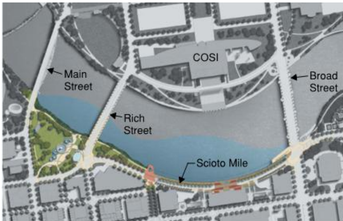
Figure 5 - The Scioto Mile plan showing the realignment of the Town Street Bridge to Rich Street. The Main Street Bridge is on the left and the Discovery Bridge on the right.
