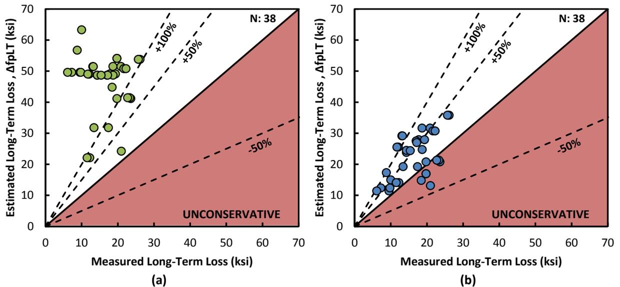
Figure 7: (a) AASHTO LRFD 2004 and (b) AASHTO LRFD 2012 estimated long-term loss vs. measured long-term loss
