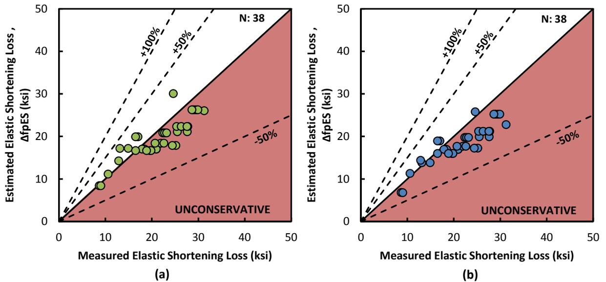
Figure 6: (a) AASHTO LRFD 2004 and (b) AASHTO LRFD 2012 estimated elastic shortening vs. measured elastic shortening
