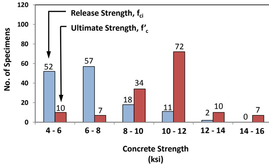
Figure 4: Release strength and ultimate strength of concrete used to construct specimens
