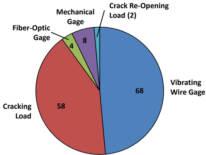
Figure 1: Method used for measuring prestress loss
