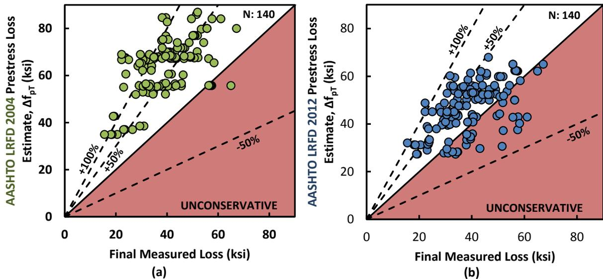
Figure 5: (a) AASHTO LRFD 2004 and (b) AASHTO LRFD 2012 prestressed loss estimate vs. final measured loss
