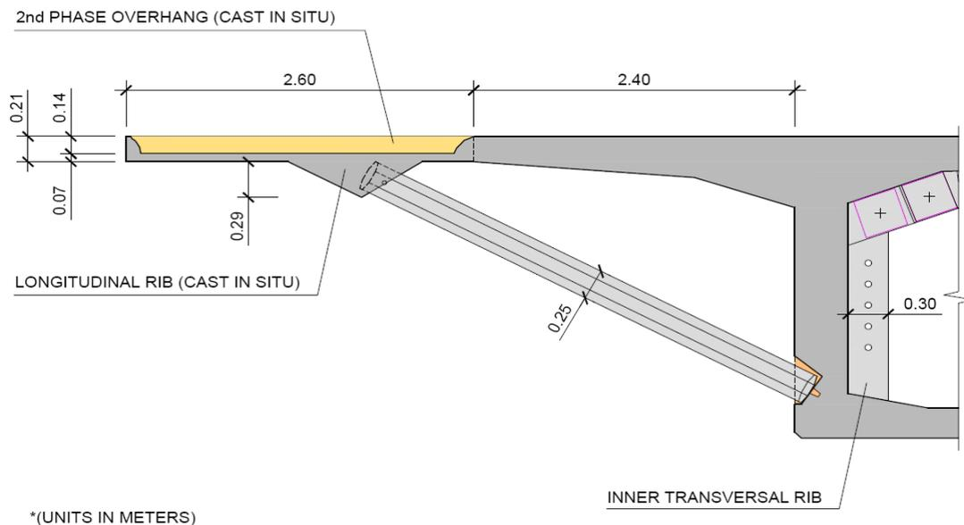
Figure 3: General Cross Section of the Deck
