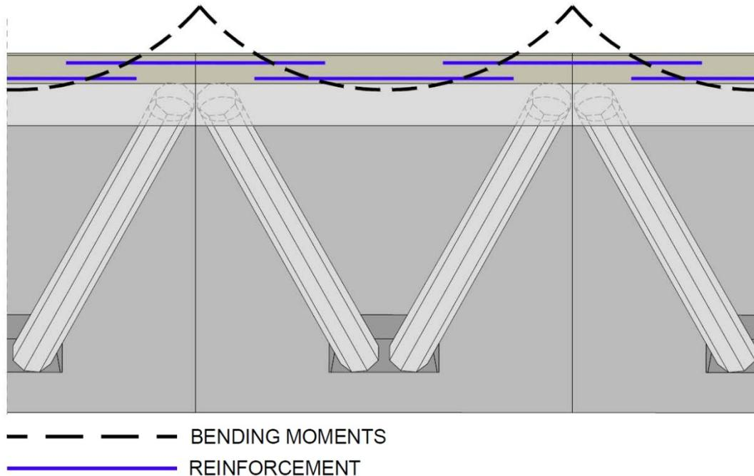
Figure 6: Longitudinal Reinforcement
