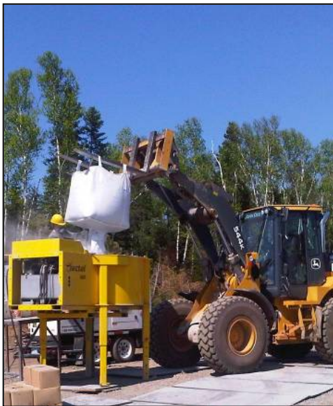
Fig. 7: Loading premix into 0.5m 3 mixers
