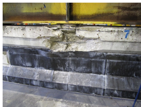
Figure 11: failure shape mode of full scale PSC beam by static testing
