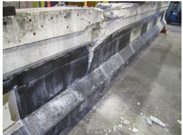
Figure 10: failure shape mode of full scale PSC beam by static testing
