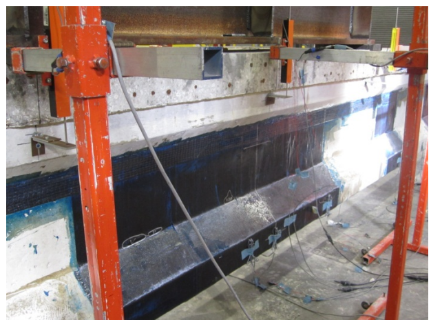
Figure 11: failure shape mode of full scale PSC beam by static testing
