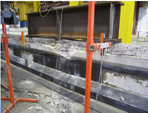
Figure 10: failure shape mode of full scale PSC beam by static testing
