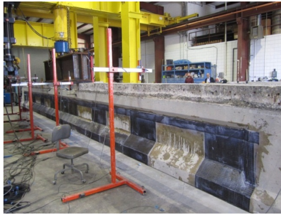
Figure 5: Full scaled girder test setup and testing
