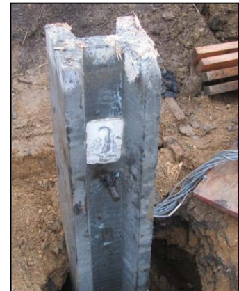
Fig. 18 Slight Damage to UW1-2 at EOD
