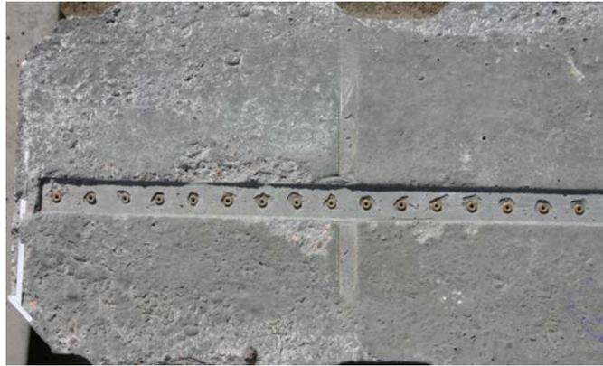
Figure 6. Metal gauge points embedded in the concrete surface to facility the transfer length measurement by the Whittemore gauge
