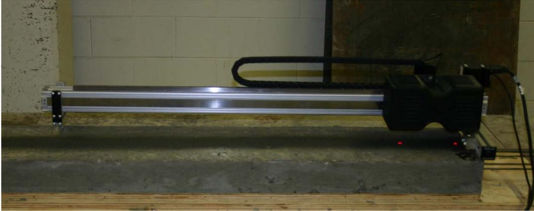
Figure 16. An automated LSI sensor positioned on a concrete prism
