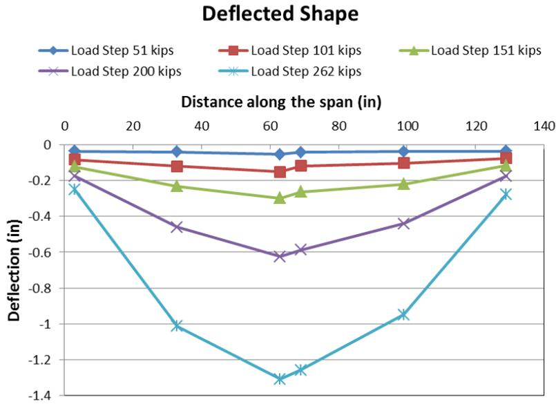
Fig. 23 Deflected shape of the specimen with straight web and extended bars for various load steps
