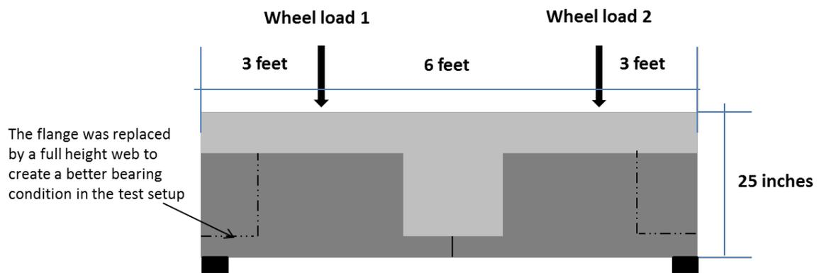
Fig. 12 Schematic representation of test setup
