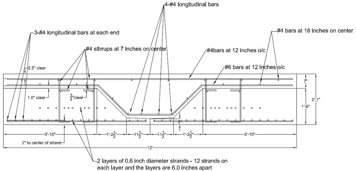
Fig. 18 Reinforcing Details for Test Specimen #4 – Tapered web cross-sectional shape with no connection
