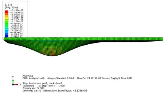
Fig. 8 Side view of the deformed shape due to live loads. Notice the effect of transverse bending on the joints between the inverted T-beams
