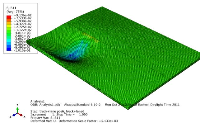
Fig. 7 An isometric view of the deformed shape due to live loads of the two span continuous bridge modeled with precast Inverted T beams and cast in place concrete topping (Finite Element Model created in Abaqus<sup>7</sup>)
