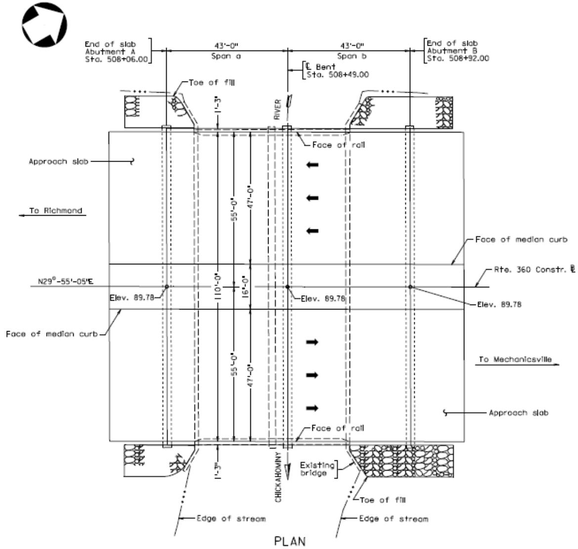
Fig. 5 Preliminary plan view of the soon to be replaced two-span continuous bridge on Route 360 over Chickahominy River (Courtesy of Virginia Department of Transportation<sup>6</sup>)
