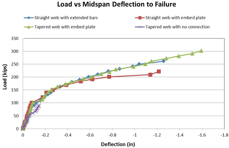
Fig. 19 Comparison of Load Deflection Curves for all four test specimens
