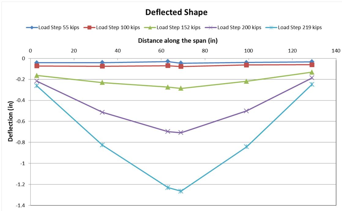
Fig. 21 Deflected shape for the specimen with the straight web and embedded plate connection for various load steps
