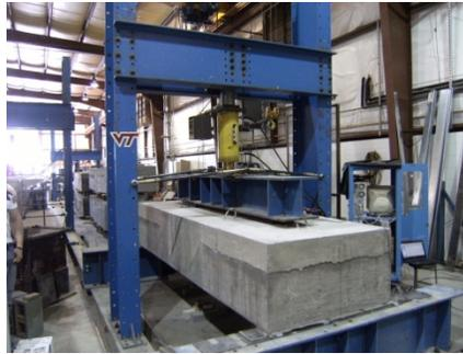
Fig. 11 Photograph of test setup showing the loading frame, load actuator, the spreader beam which loads the specimen at ¼ points and the two steel support beams which provide 6 in. bearing on each side.
