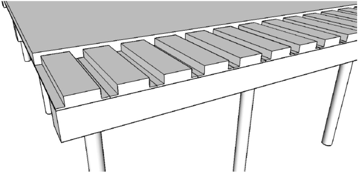
Fig. 1 Precast Inverted T-beam System
