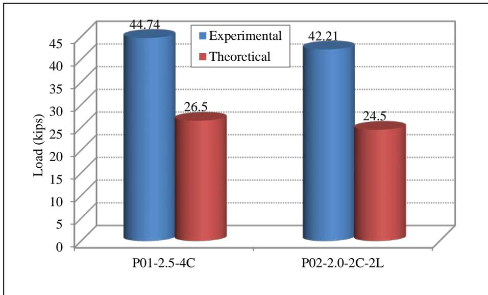
Figure 14. Experimental versus theoretical failure loads
