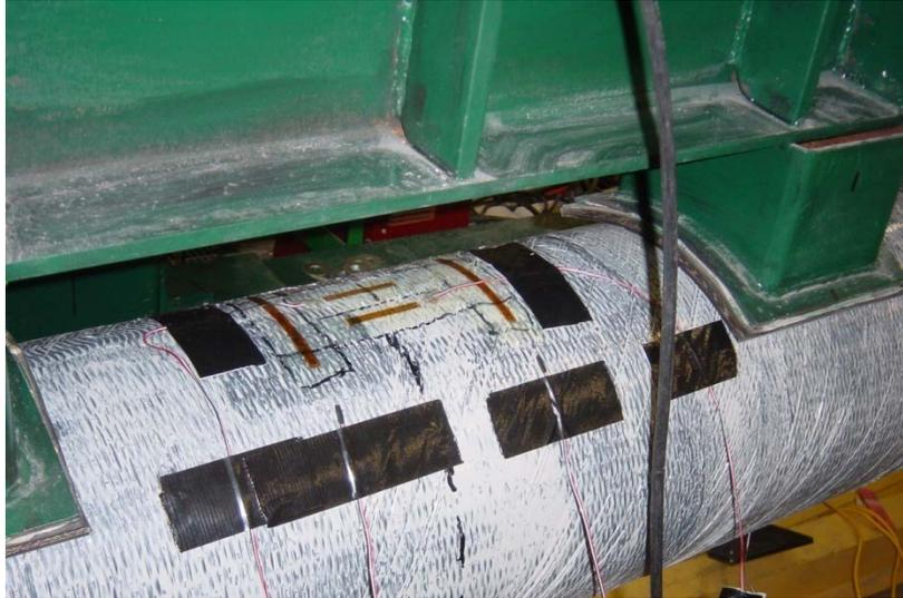
Figure 5. Location of compression set of strain gages
