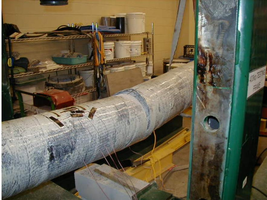
Figure 11. Failure mode of pole P01-2.5-4C, wrapped in one direction
