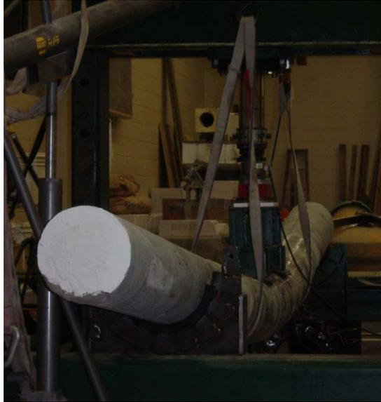
Figure 13. Deflection of pole P01-2.5-4C, wrapped in one direction, just before failure
