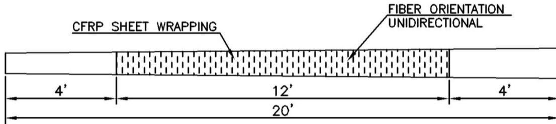
Figure 1. Wrap length and circumferential carbon fiber orientation (specimen P01-2.5-4C)
