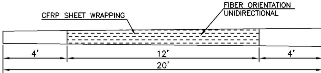
Figure 2. Wrap length and longitudinal carbon fiber orientation (specimen P02-2.0-2C-2L)
