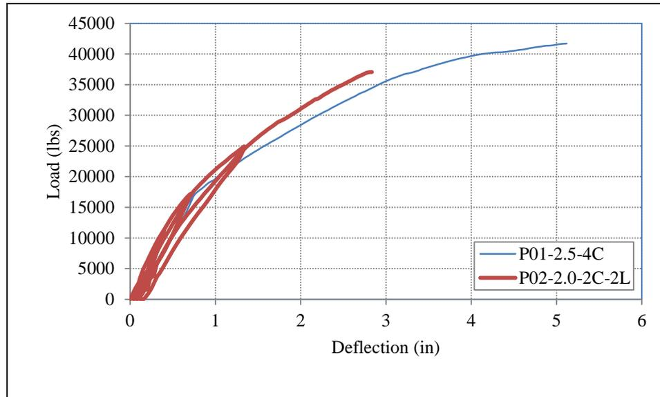
Figure 7. Load-deflection curve for the specimens
