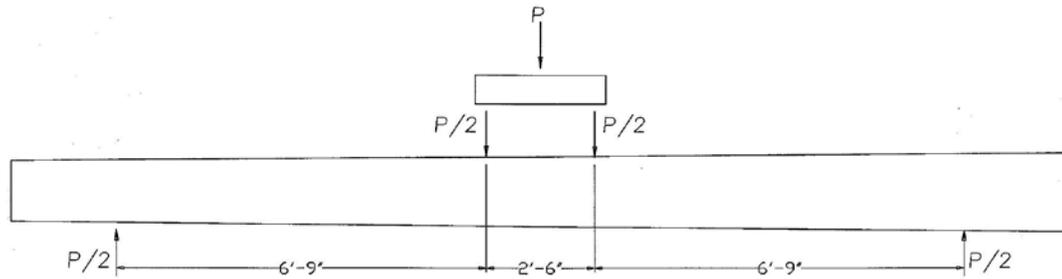
Figure 3. Schematic diagram of test setup
