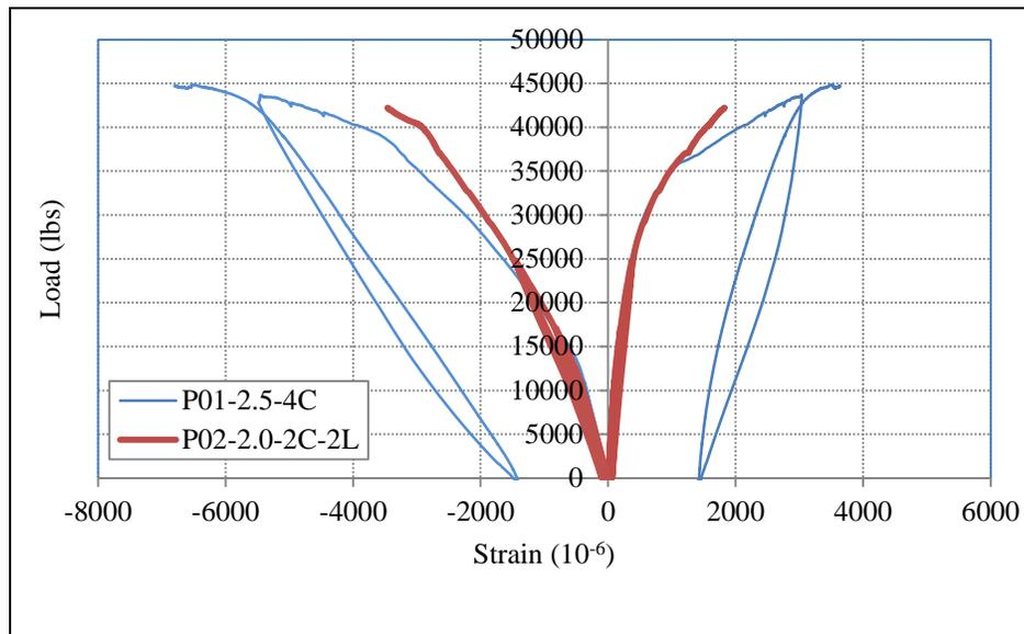
Figure 10. Load versus strain for the tested poles
