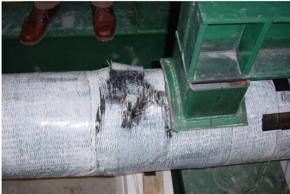
Figure 12. Failure mode of pole P02-2.0-2C-2L, wrapped in two directions
