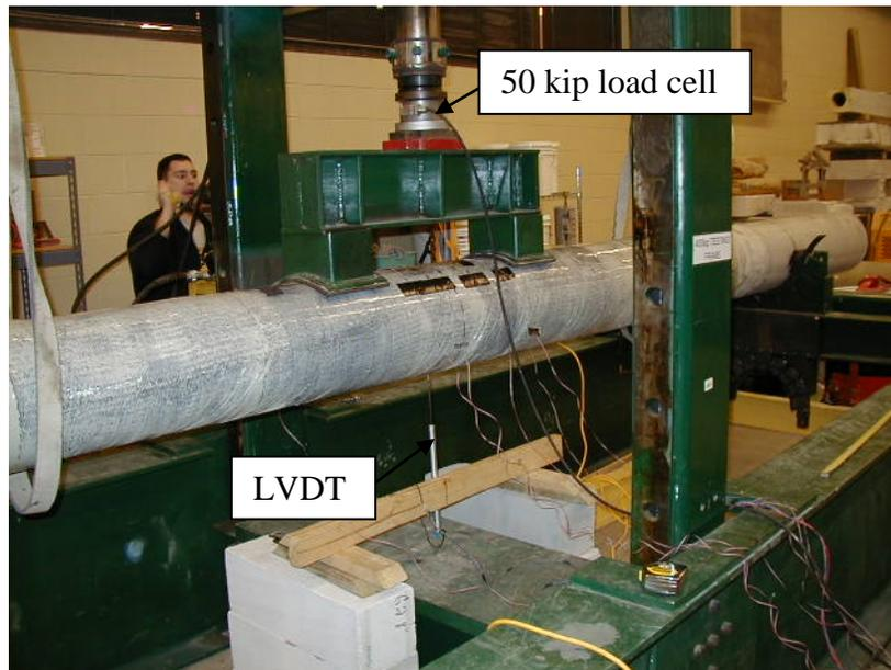
Figure 6. Location of the LVDT and the load cell
