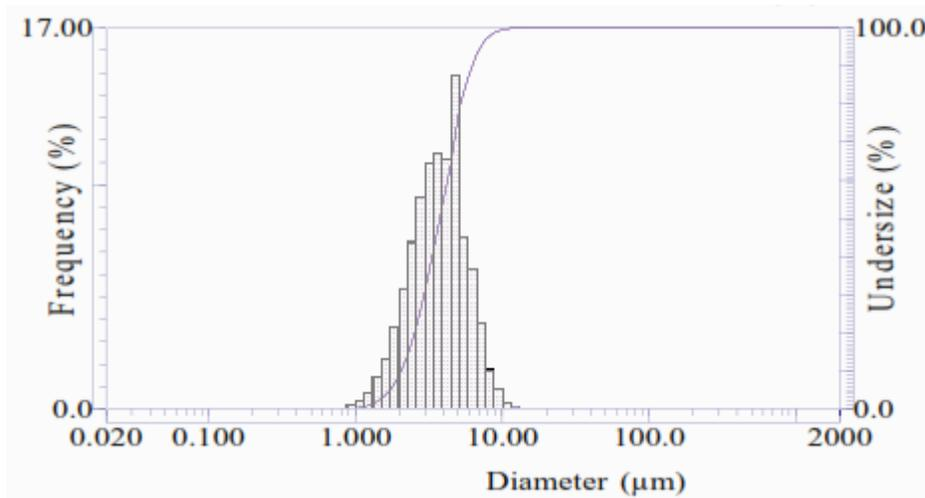
Fig. 3 Particle Size Distribution of “Ultrafine” Pumice
