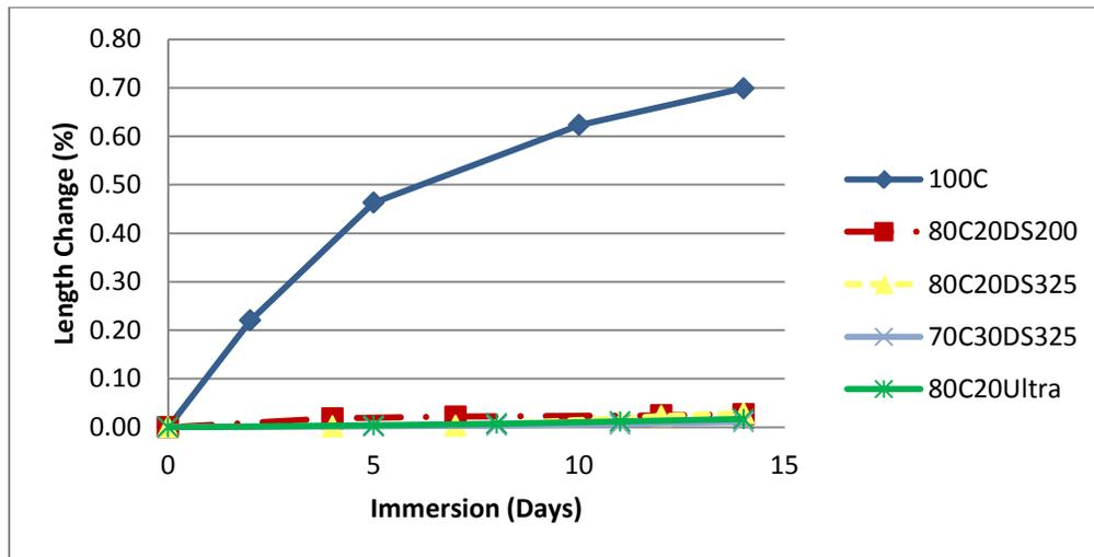
Fig. 10 Length Change (%) of Mortar Specimen due to ASR
