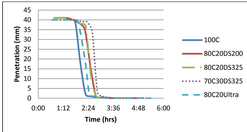
Fig. 7: Penetration resistance of different mixtures
