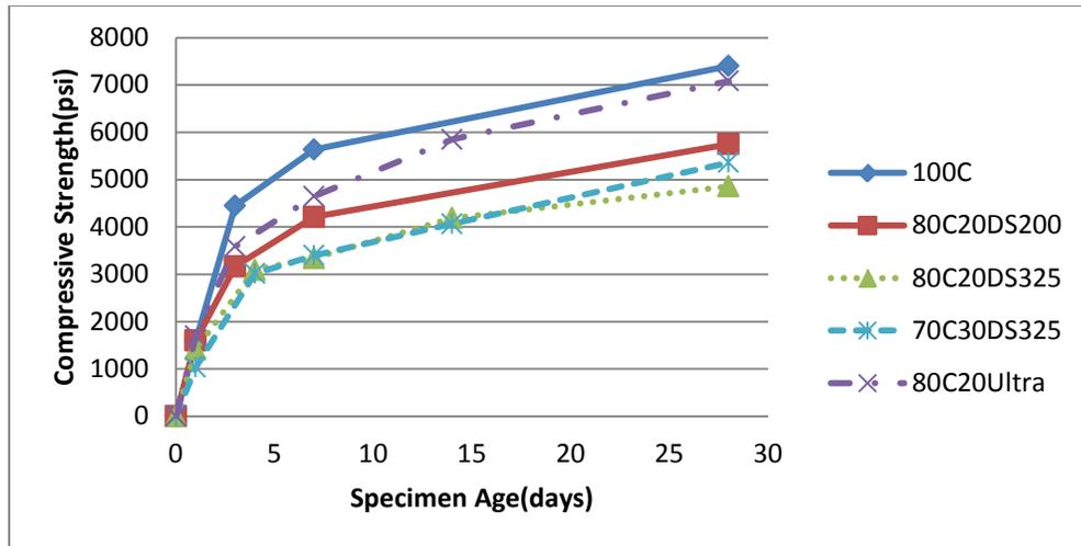
Fig. 8 Compressive strength for 4X8 cylinders
