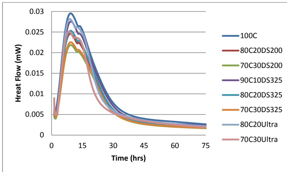
Fig. 4 Heat Flow for different mixture combinations during first 75 hours
