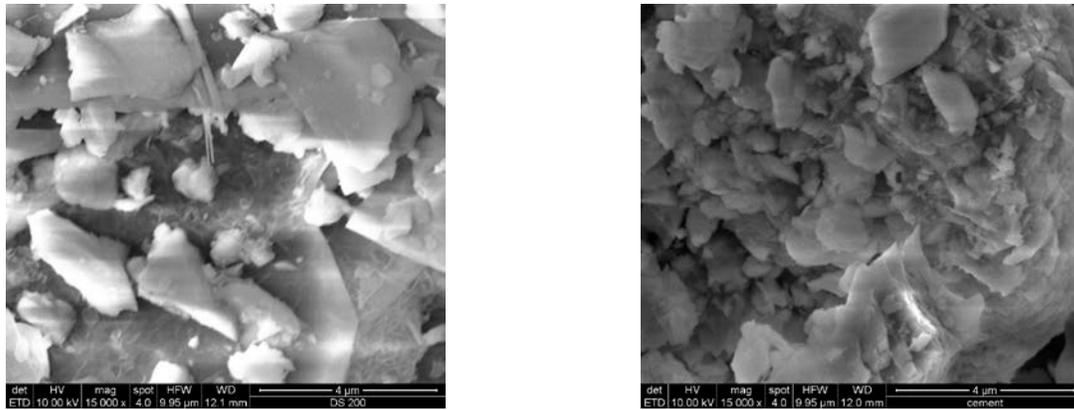
Fig. 2 Scanning Electron Micrograph for DS200 and Cement @ 2000X and 1500X
