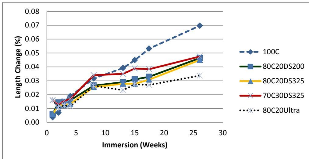
Fig. 9 Length Change (%) of Mortar Specimen due to sulfate
