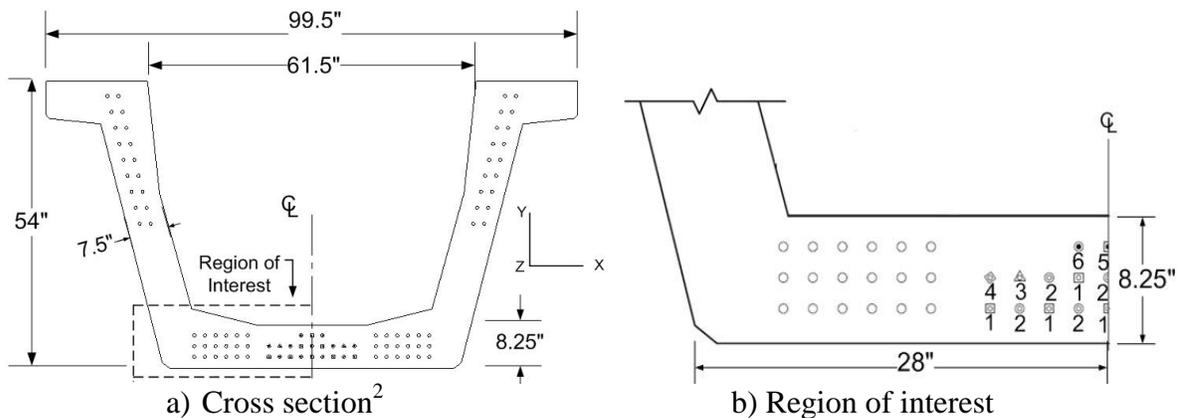
Fig. 3 U-beam: Cross section and region of interest for FE model<sup>9</sup>
