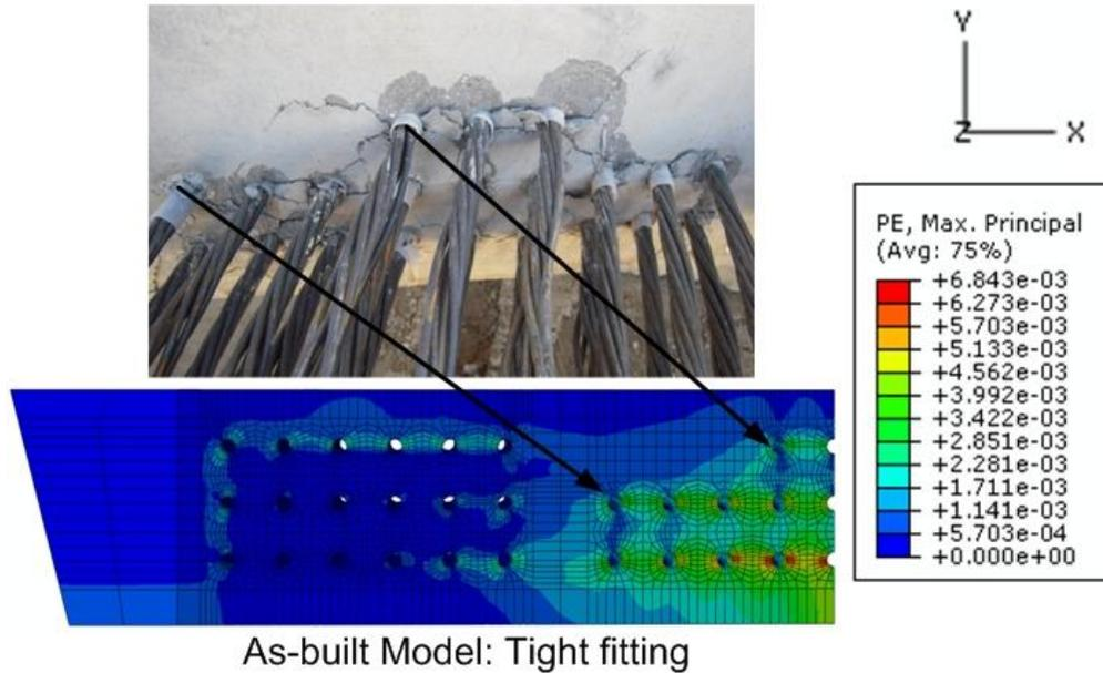
Fig. 7 Observed damage and maximum principal plastic strains for as-built U-beam model
