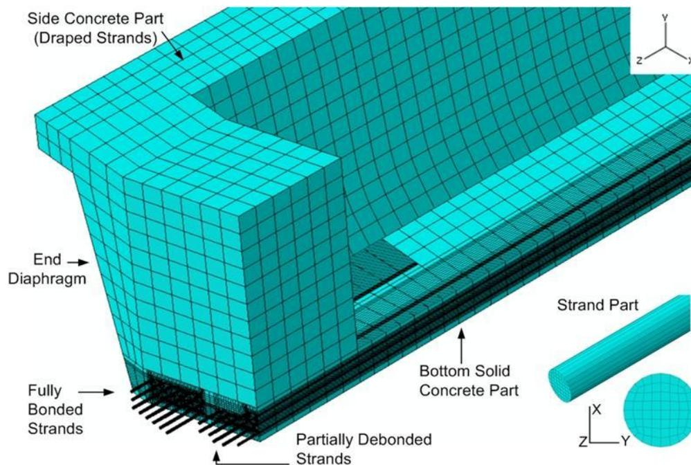
Fig. 5 View of as-built U-beam FE model
