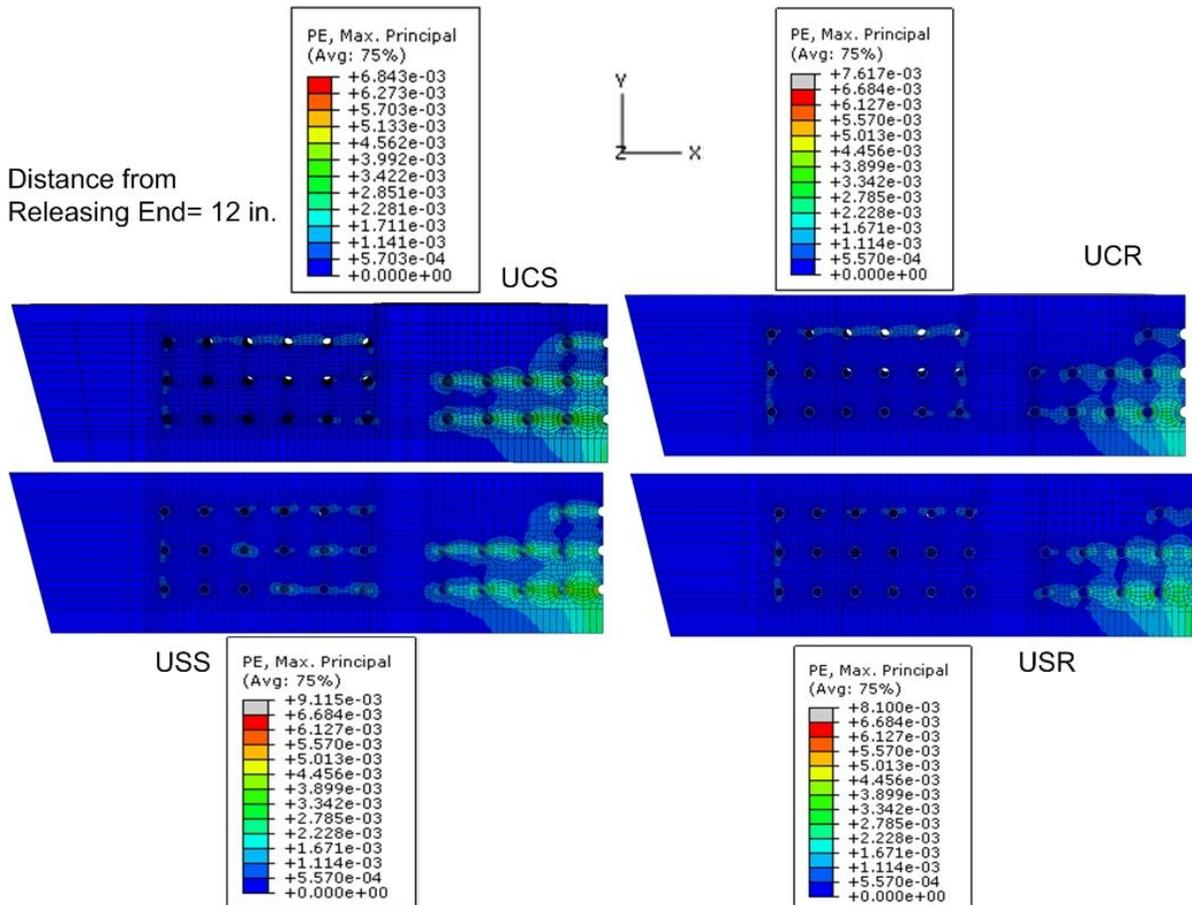
Fig. 8 Maximum principal plastic strains for U-beam models 12 in. (305 mm) from beam end
