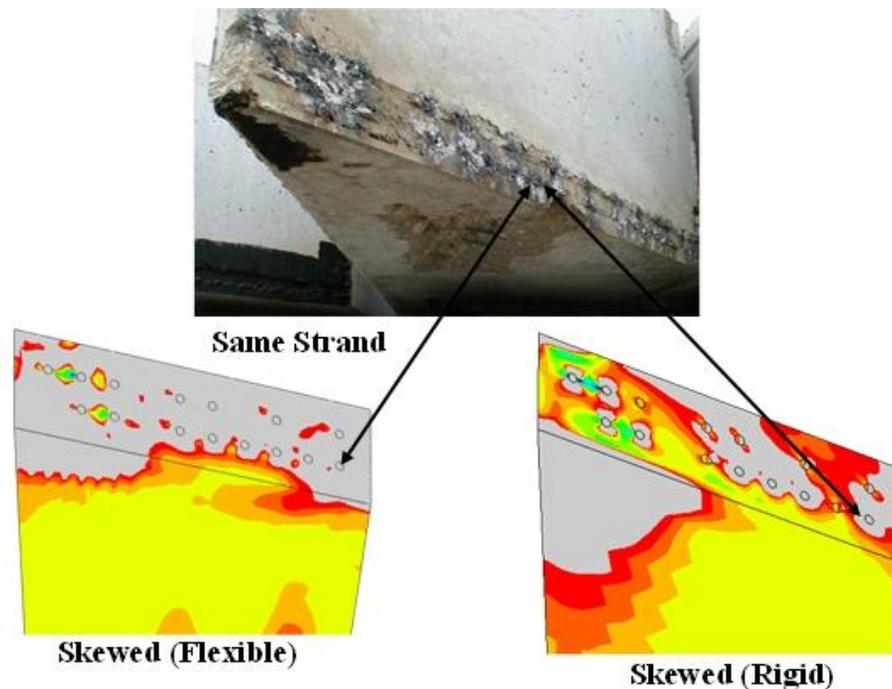
Fig. 6 Observed and predicted damage for the Box-beam case studies
