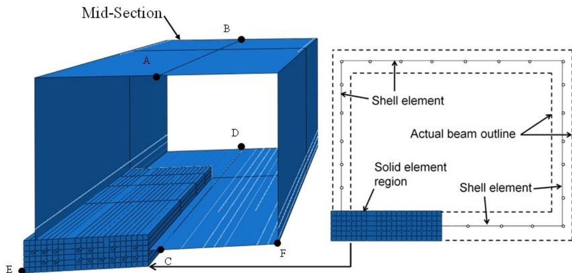
Fig. 4 View of Box-beam FE model and region of high interest
