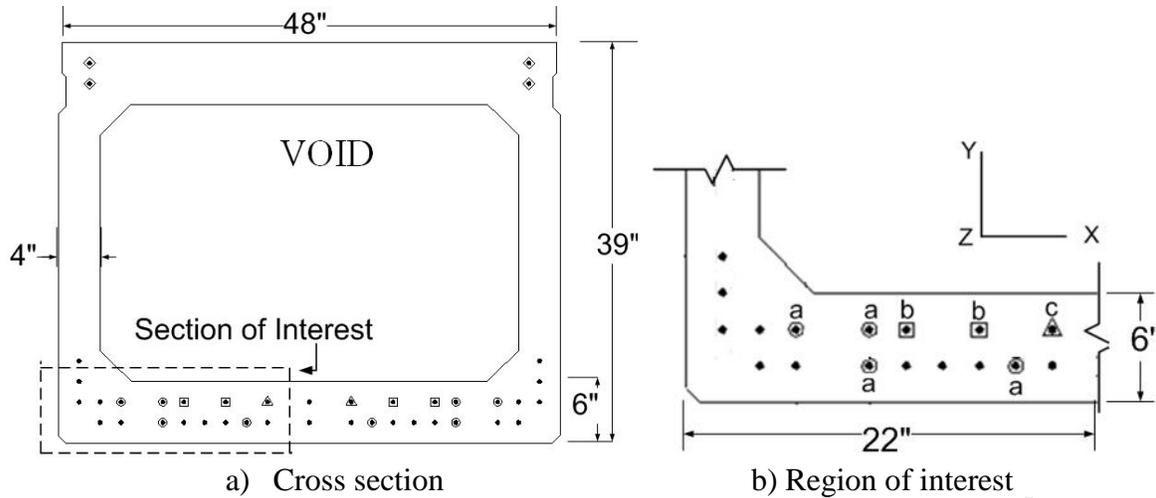
Fig. 2 Box-beam: Cross section and region of interest for FE model<sup>7</sup>
