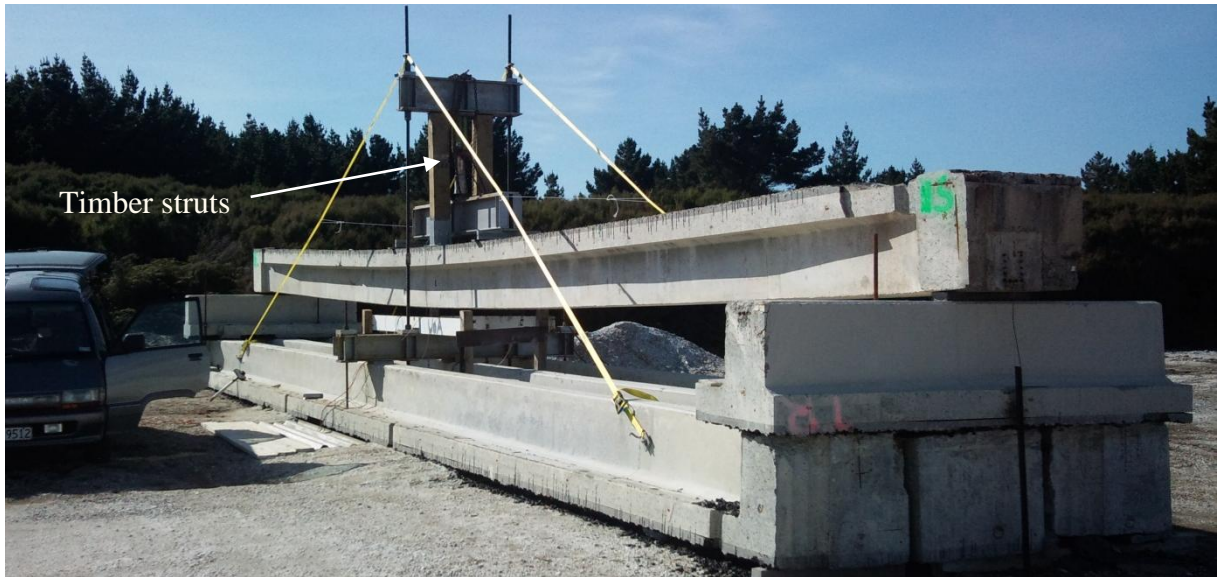
Fig. 9: Test rig and deflected beam 4C
