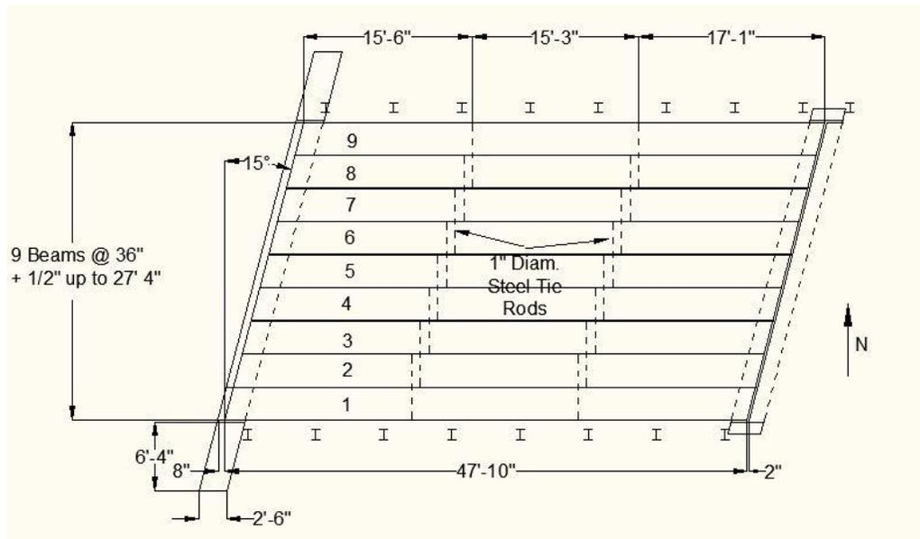
**Figure 2: FAY 35-17-6.82 Bridge Span**
