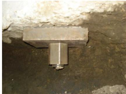
**Figure 5: Abutment Test Frame Anchorage**
