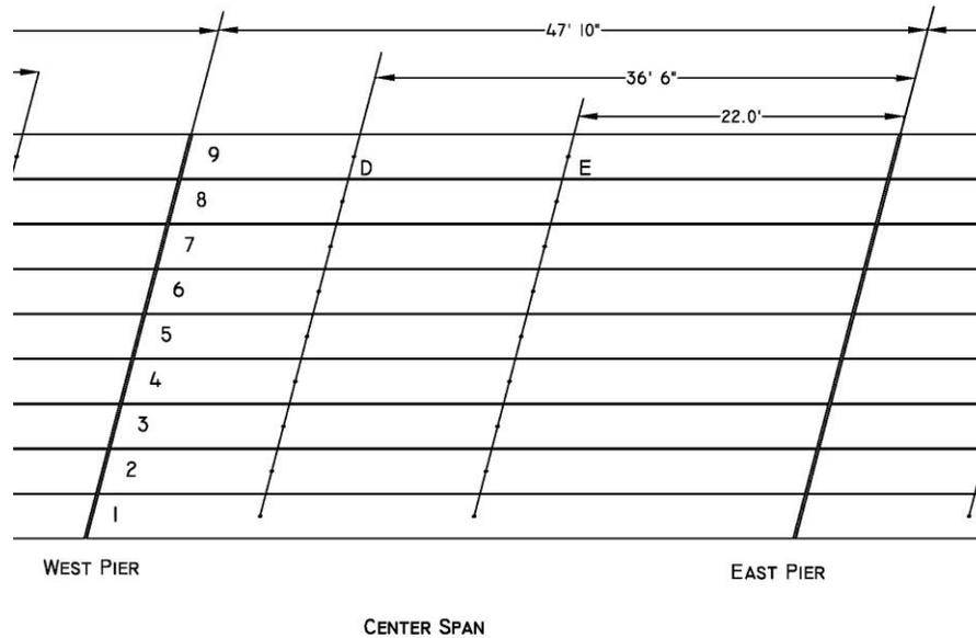
**Figure 10: Instrumentation Locations for Center Span**
