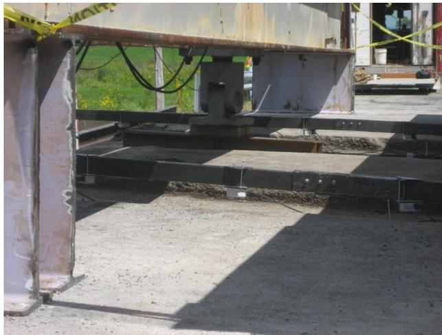
**Figure 9: Steel Tubes with String Potentiometers**
