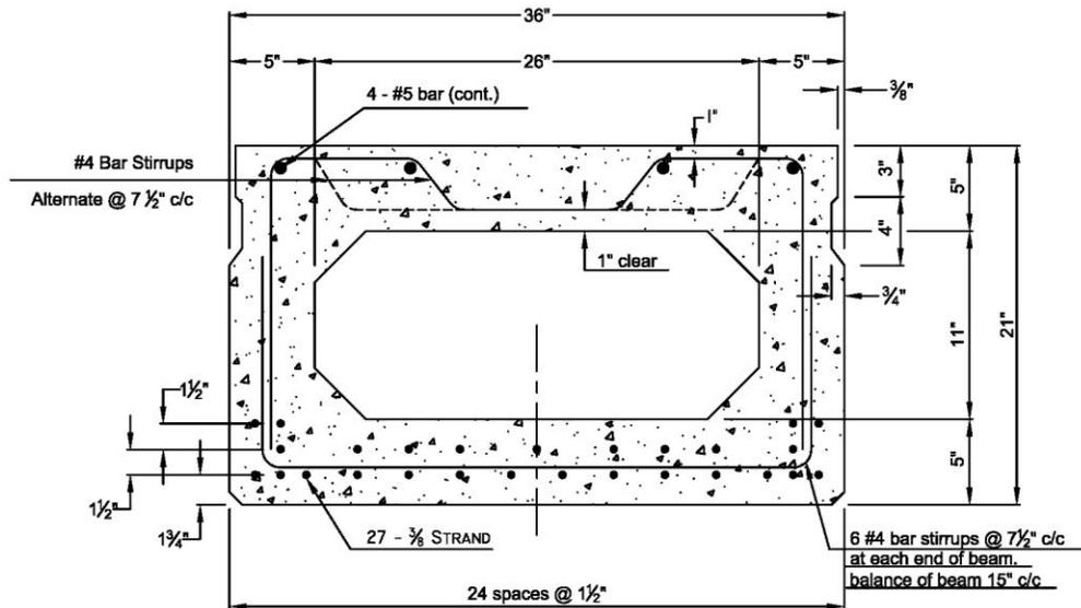
**Figure 3: FAY 35-17-6.82 Beam Section**
