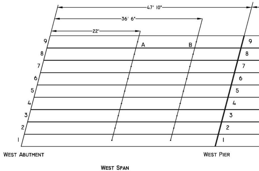
**Figure 12: Instrumentation Locations for West Span**
