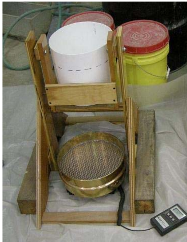
Fig. 2 Sieve stability test apparatus
