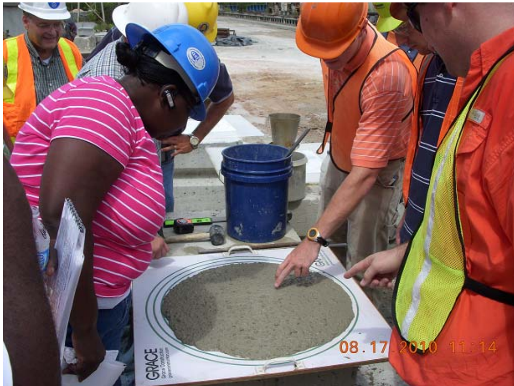
Fig. 5 Slump flow and VSI training of ALDOT and Hanson Precast personnel
