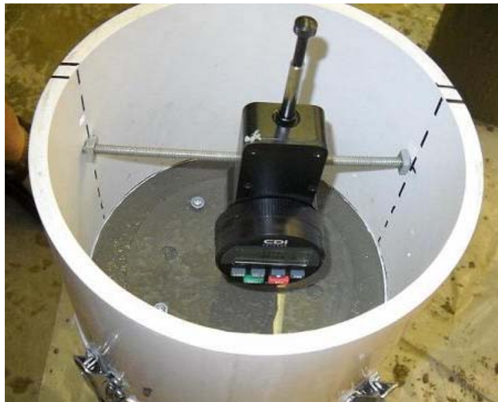
Fig. 3 Surface settlement test apparatus with clear acrylic plate
