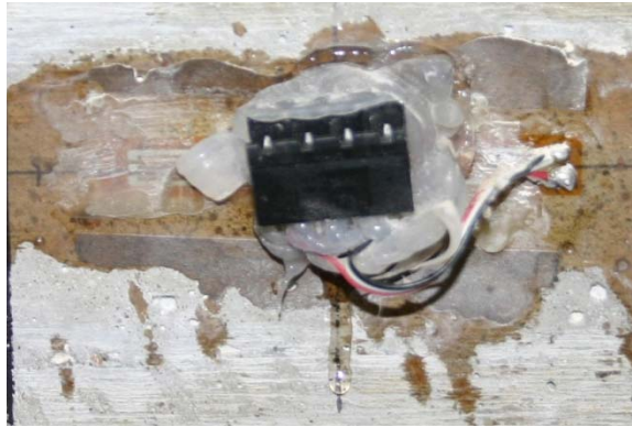
Fig. 3 Strain Gage with Terminal Block Mounted Using Silicon
