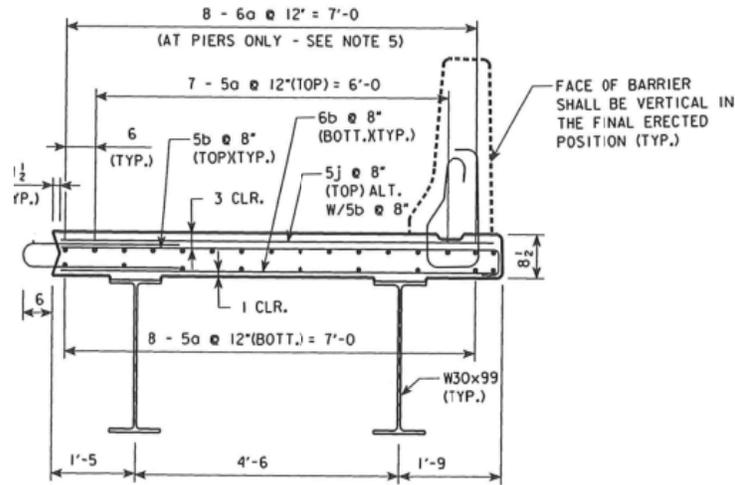
Figure 8. Section through exterior superstructure module
