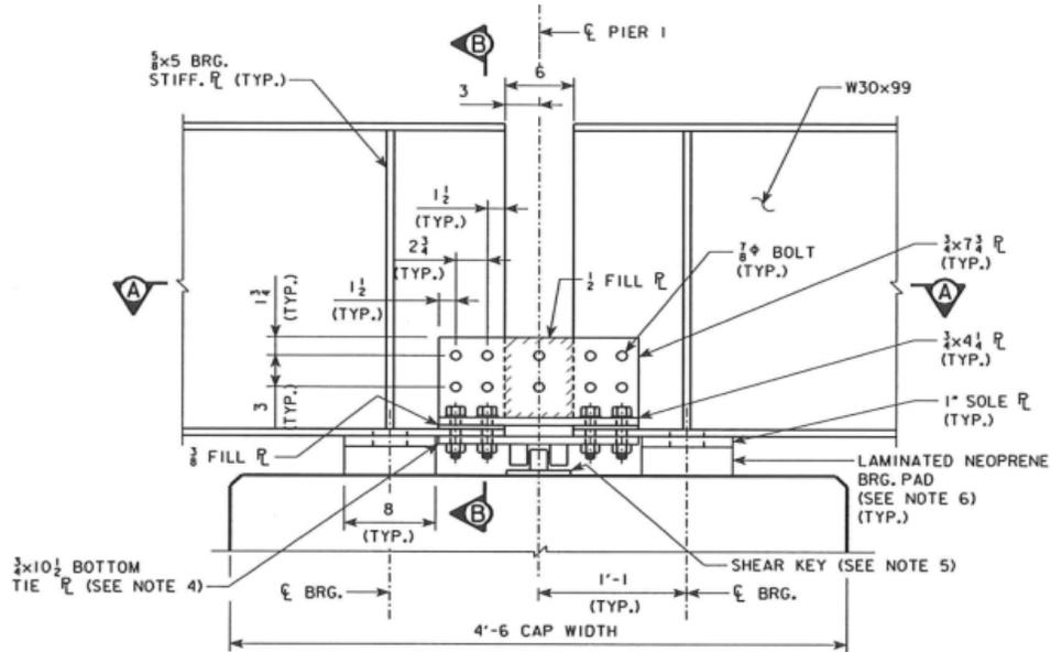
Figure 9. Structural steel connection between adjacent spans
