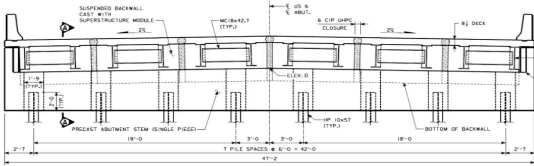
Figure 3. Typical section through precast abutment backwall
