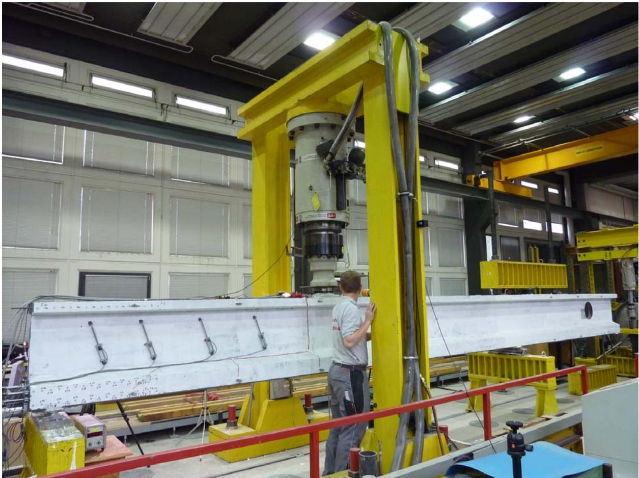
Figure 7: Test setup of the shear tests with 70 cm (27.6 in) height (1<sup>st</sup> test setup)
