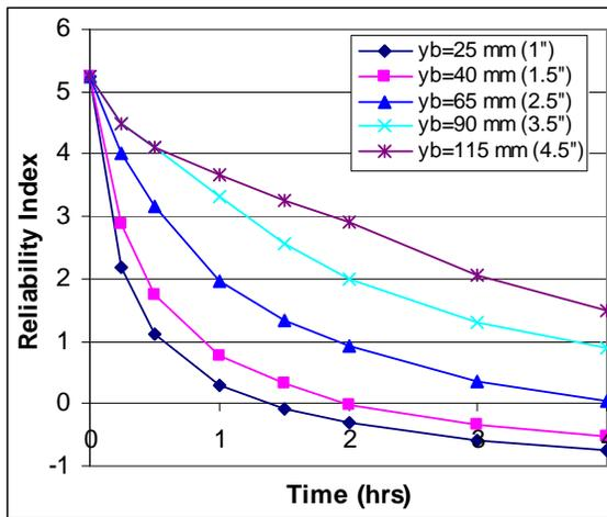
Fig. 5. Effect of Concrete Cover, Base Beam 1
