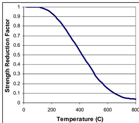
Fig. 2. Prestressing Steel High-Temperature Strength Reduction Factor
