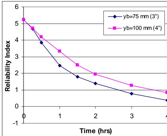
Fig. 6. Effect of Concrete Cover, Base Beam 2
