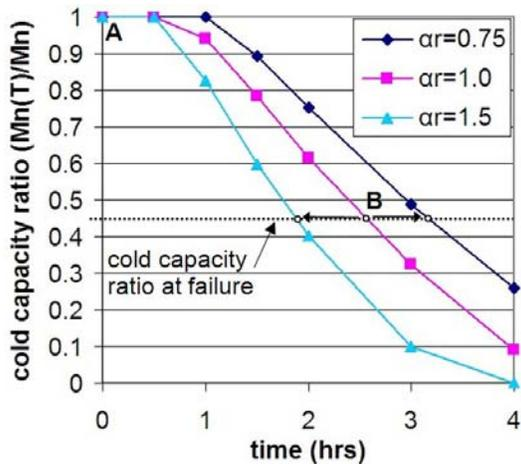
Fig. 3. Effect of Thermal Diffusivity in the Wickstrom Model
