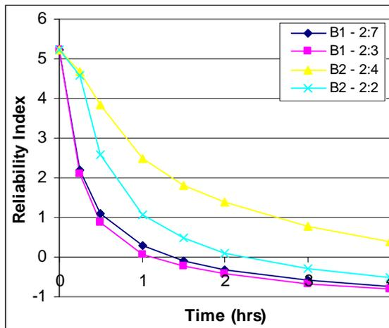
Fig. 7. Effect of Proportion of End Strands to Total Strands Per Layer
