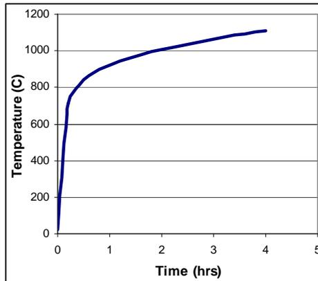
Fig. 1. Standard Fire Time-Temperature Curve
