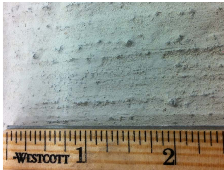
Figure 11. Photograph of bottom block of specimen WET-LBX-2 before placement of top block concrete. This photograph was taken after brushing the surface and blasting the surface with compressed air.
