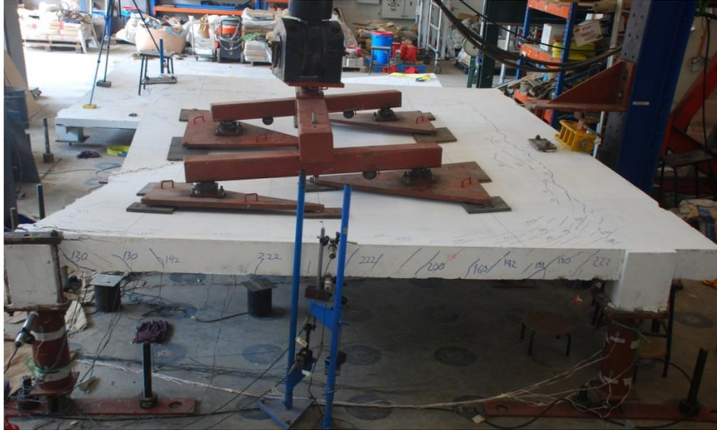
Fig. 8 Failure Mode of Specimen PE-02 SA
