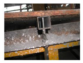
The combination of a linear axle surface with some adjustment in its height and the ideal cover that accepted the required shapes depending on the form adjustment, the 3D form resulted in a adjustable casting bed with unique features for the project: it gave us the possibility to adjust shapes in much less time instead of producing a new mold with impressive cost and time savings.
