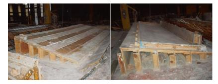
In a regular production system, the decision would be to use wood molds, where some simple adjustments solved a typical low repetition, however the shop tickets indicated that each panel was different. To manufacture molds with 296 different variations for a single piece use would be totally ineffective.
