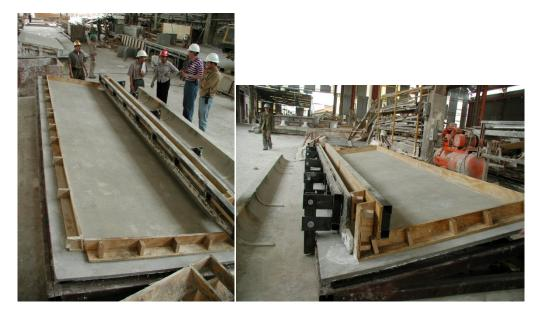
We had to seek the way to manufacture "disposable" inexpensive molds that did not require so much time to manufacture or to design a master molding system that we could adjust to the given requirements: one mold for all.
