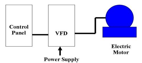
Fig. 1: The Simplicity of Control Set-up
