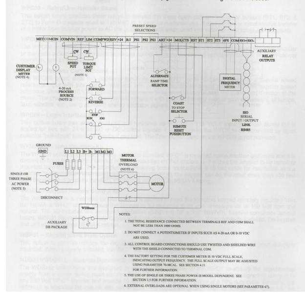
Fig. 2:Typical Variable Frequency Drive Hook-up (Reprinted with permission Vacon, Inc.)
