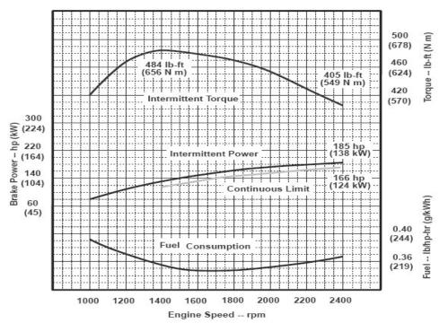
Fig 3: Typical diesel engine torque curve (Reprinted with permission of Frontier Power)
