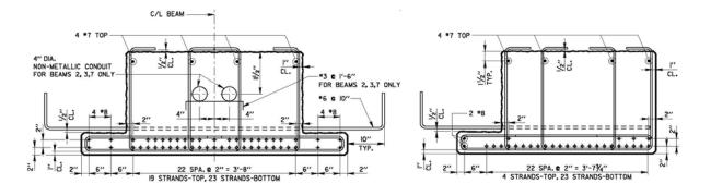
Fig. 11. (a) Interior Beam Section.
