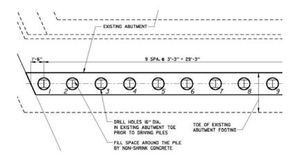
Fig. 7. Abutment Piling Plan.
