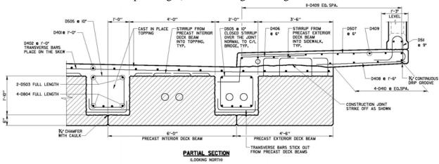
Fig. 10. Superstructure Partial Section.
