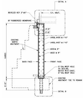
Fig. 6. Typical Abutment Section.
