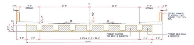
Fig. 3. Bridge Typical Section
