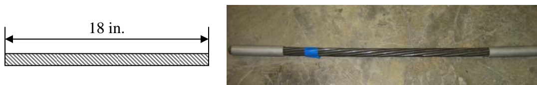
Fig. 3 – Schematic and Actual View of Coupon Specimens
