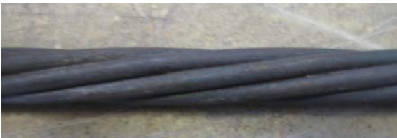
Fig. 10 – Strand after Exposure to 1000°F (538°F)
