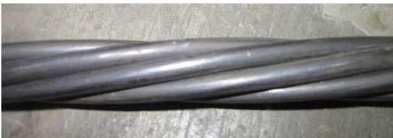
Fig. 9 – Strand after Exposure to 800°F (427°C)
