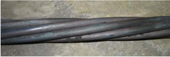
Fig. 12 – Strand after Exposure to 1300°F (704°C)
