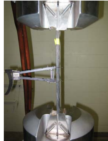
Fig. 7 – Tension Test setup
