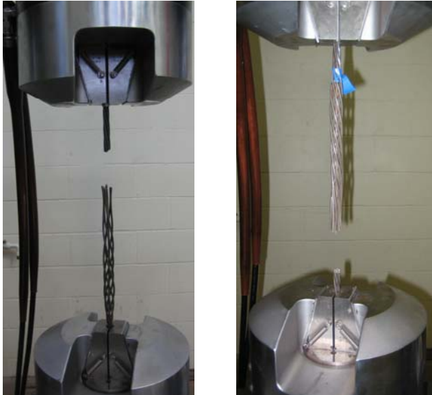
Fig. 14 – Typical Failure Mode of Prestressing Strand in Tension
