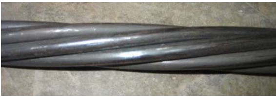
Fig. 8 – Strand after Exposure to 500°F (260°C)
