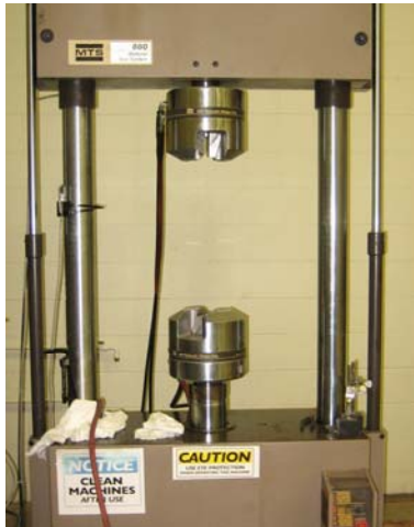
Fig. 6 – MT880 Testing Machine Prior to Tension Tests
