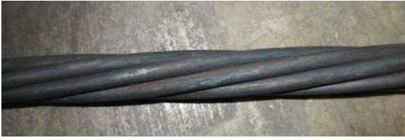
Fig. 11 – Strand after Exposure to 1200°F (649°F)
