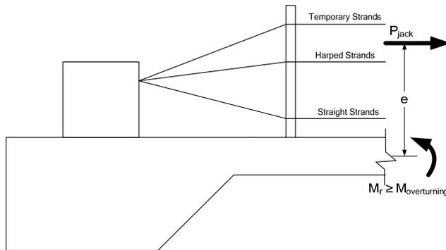
**Figure 1 Free Body Diagram of Critical Section of Prestressing Line**
