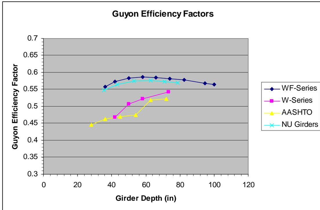
Figure 4 Girder Efficiency Comparison (Ref. 8)
