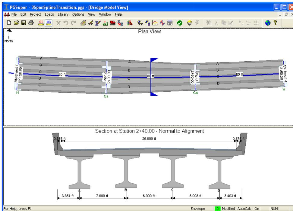
**Figure 2 Complex Bridge Modeled with PGSuper**
