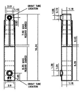
Figure 7. Grout Filled Mechanical Splicer for # 9 bars
