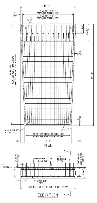
Figure 4. Trapezoidal Precast Footing Segment, Type 16 F
