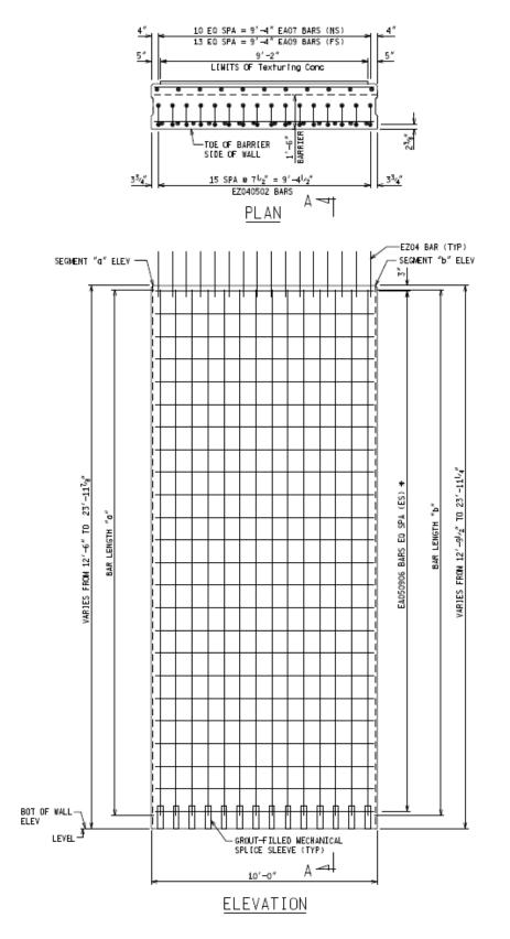
Figure 6. Precast Wall Stem Segment, Type 3 W
