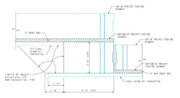
Figure 5. Precast Footing Block Elevation
