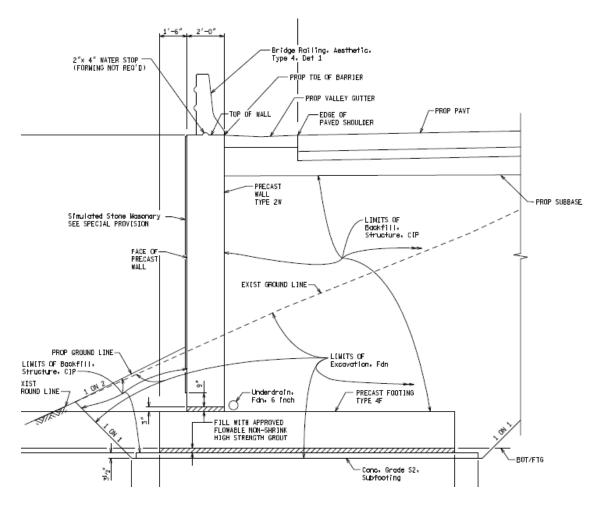
Figure 2. Precast Cantilever Retaining Wall System
