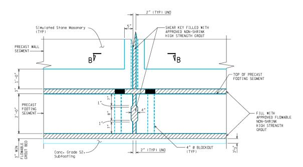
Figure 8. Vertical Shear Keys Detail
