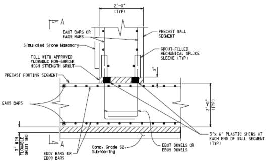
Figure 3. Typical Wall Segment-to-Footing Segment Connection
