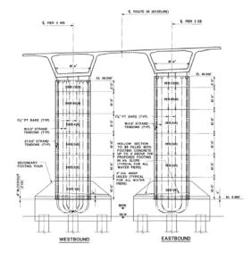
Fig. 4 Precast Piers Elevation
