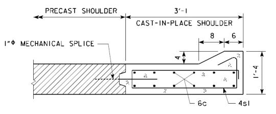
Figure 10 (Cross section of gutter-line with cast-in-place section)
