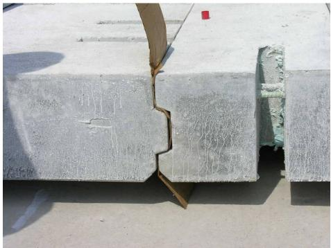
Figure 14 (Fit-up test at shoulder line keyway)
