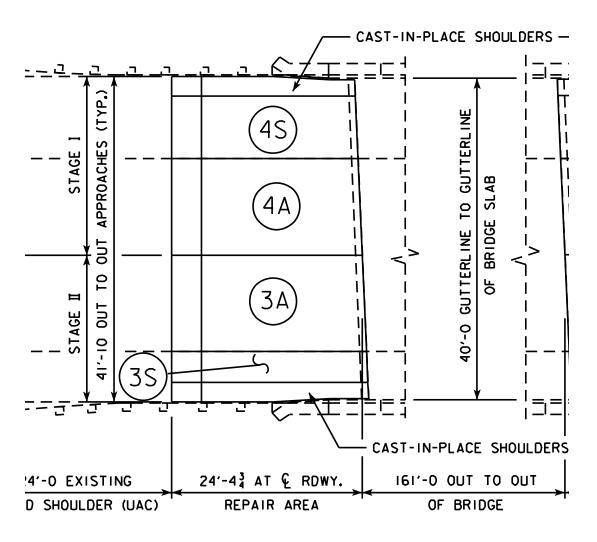
Figure 6 (Plan view of abutment showing individual panels)
