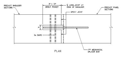
Figure 9 (Typical shoulder line connection of precast panels)
