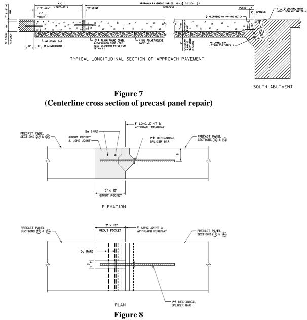
(Typical centerline connection of precast panels)
