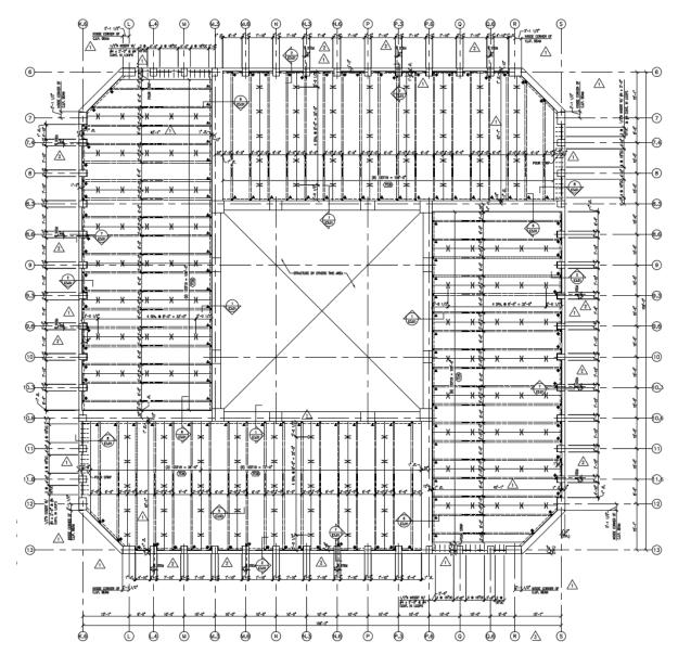
Figure 2 Double Tee Framing Plan - Tower
