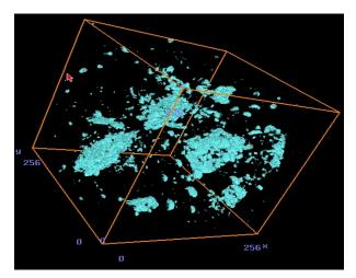
**Figure 1: THREE-DIMENSIONAL X-RAY MICROTOMOGRAPHY** 1-Day Hydration
