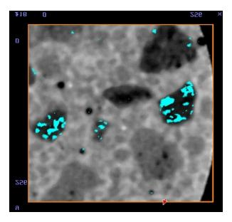
**Figure 2: THREE-DIMENSIONAL X-RAY MICROTOMOGRAPHY** 2-Day image with water evacuated regions
