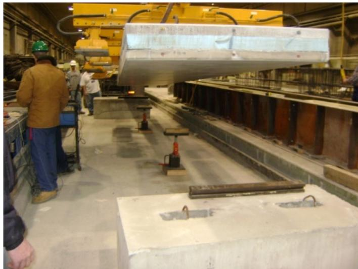
Fig. 7: End roller supports and temporary middle supports of the test specimen
