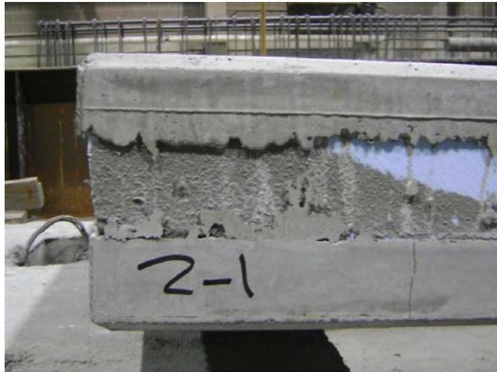
Fig. 12: Movement of top wythe relative to bottom wythe in Panel 2-1
