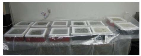
Figure 3 Ponding of Specimens
