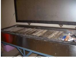
(a) Freezing-and-Thawing Apparatus
