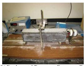
(b) Fundamental Transverse Frequency Test
