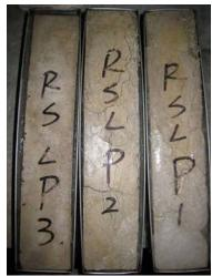
Figure 9 Failure of RSLP Mix 2 Specimens
