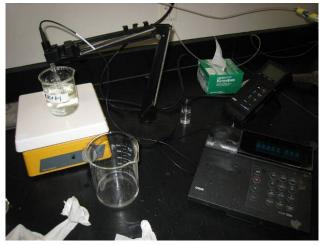
Figure 6 Chloride Concentration Determination with ISE
