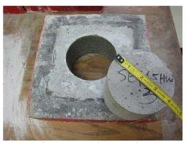
Figure 4 Specimen coring
