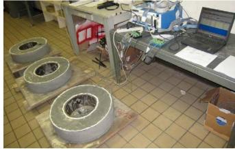
Figure 10 AASHTO PP34 Test Setup
