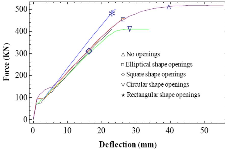
Fig. 6 Load-deflection plots of strengthened slabs with various opening shapes
