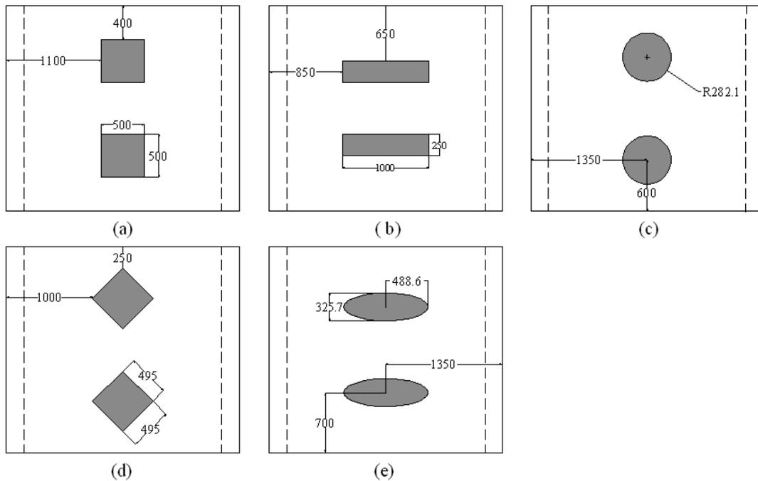
Fig. 3 Location, geometry and dimensions of openings for: (a) square; (b) rectangular; (c) circular; (d) diamond; and (e) elliptical openings (mm)
