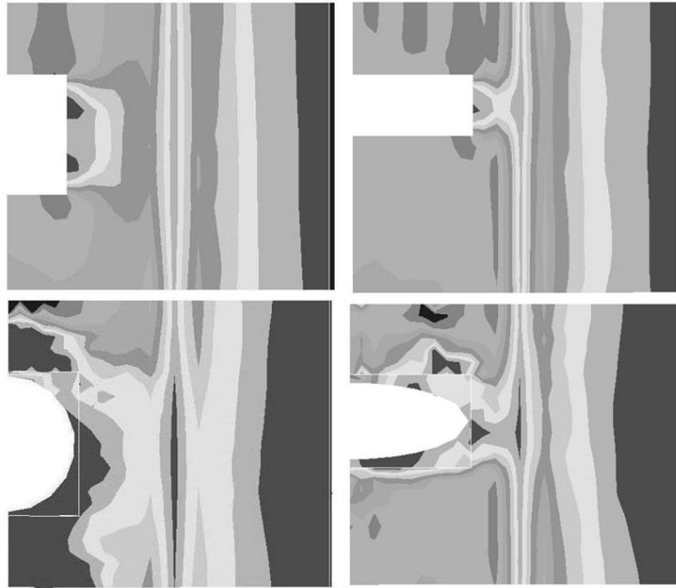
Fig. 7 Stress contours of a quarter of slab models with various opening shapes
