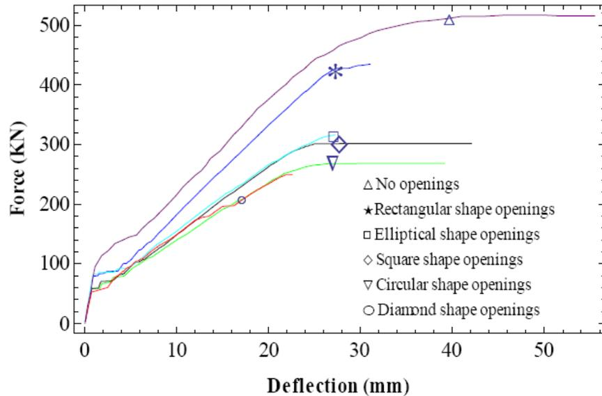
Fig. 5 Load-deflection plots of as-built slabs with various opening shapes
