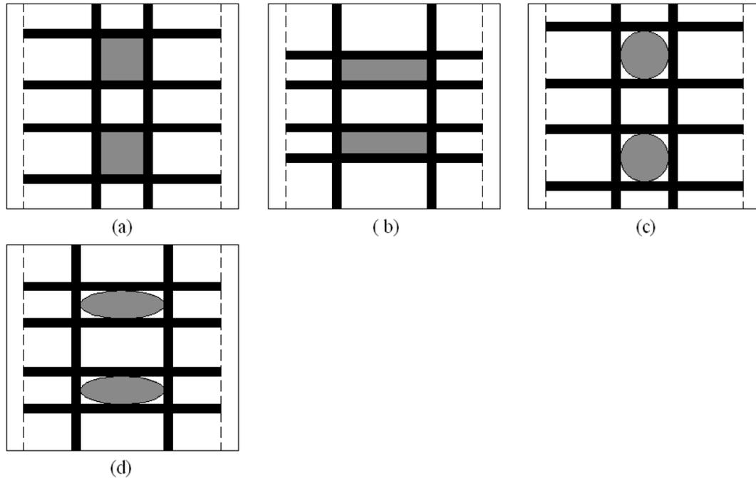
Fig. 4 CFRP reinforcement layout for: (a) square openings; (b) rectangular openings; (c) circular openings; and (d) elliptical openings
