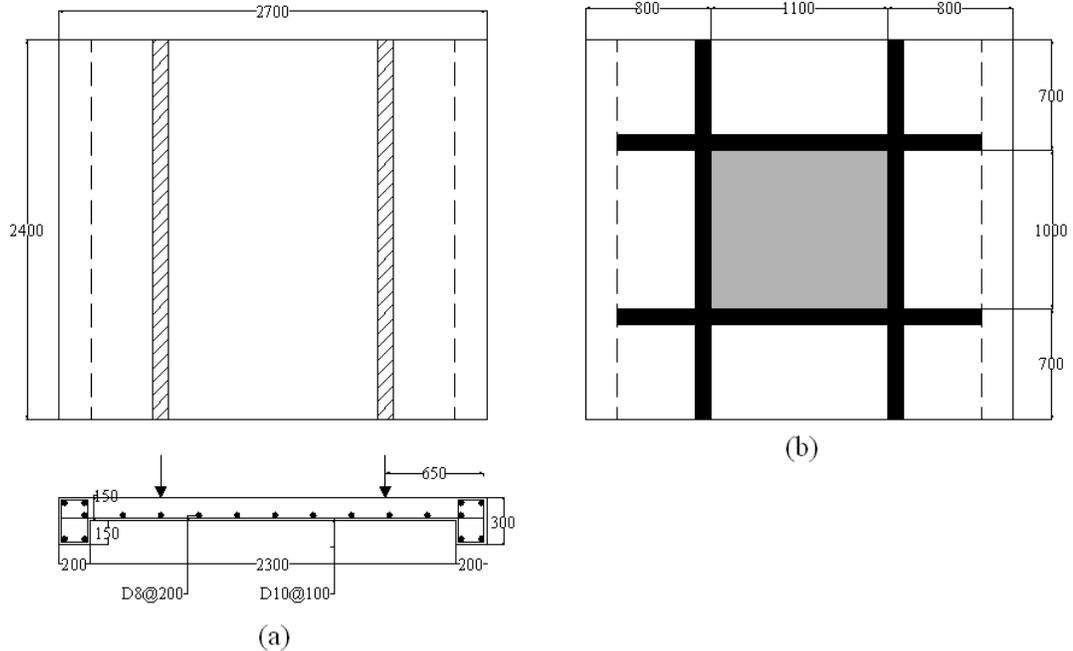
Fig. 1 Slab details of FE validated model (a) geometry, reinforcement details, and loadings position; (b) CFRP reinforcement layout (mm)
