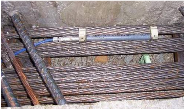
Figure 14. PT strand vibrating wire gage to measure strand force during tensioning operation and to subsequently measure deck strain after bridge construction.
