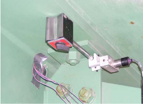
Figure 1. Displacement and foil strain sensors used to evaluate connection structural response
