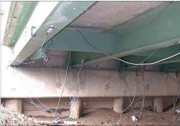
Figure 2. Multiple BDI strain sensors on bridge girders for load rating test
