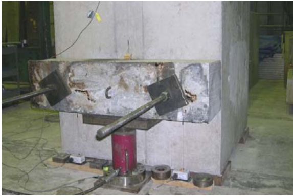
Figure 23. Laboratory test set-up of precast paving notch system
