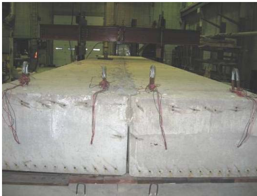
a. Girders with the shear key cast.
