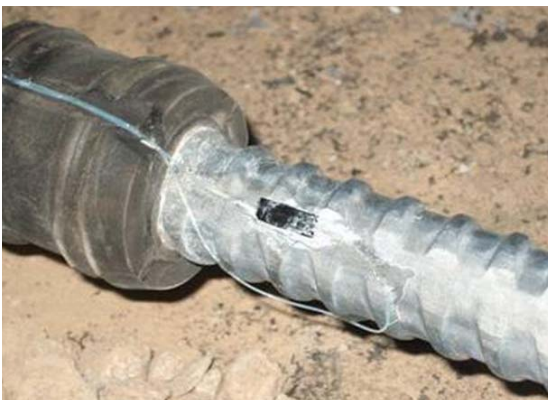
Figure 3. Uncoated fiber on hanger rod with sensor (in black package) bonded to the specimen. The actual fiber optic sensor within the fiber is extremely small (designated by arrow pointing to blue region)
