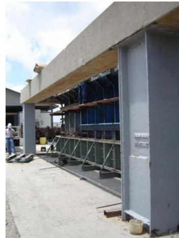
Fig. 10 Compression frame for haunched girder pre-tensioning
