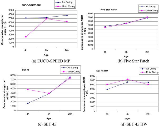
Fig. 2 Compressive Strength Development of Neat Grouts
