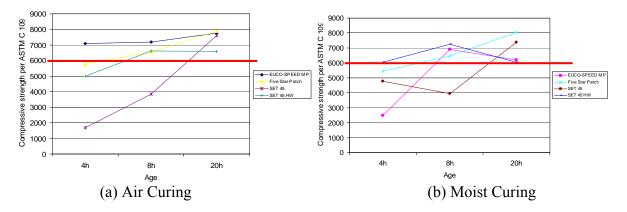
Fig. 4 Compressive Strength Development of the Neat Grouts Per ASTM C109
