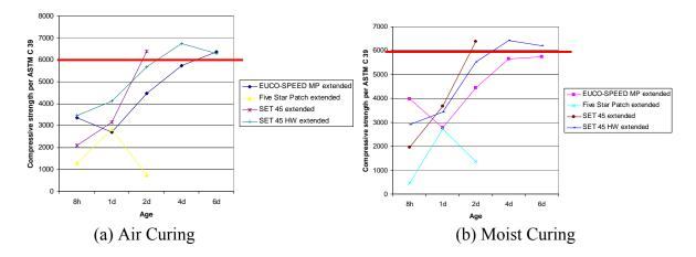
Fig. 5 Compressive Strength Development of the Extended Grouts Per ASTM C39
