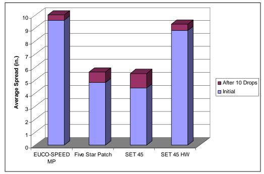
Fig. 8 Truncated Flow Cone Spread Values per ASTM C 1437 for neat gouts
