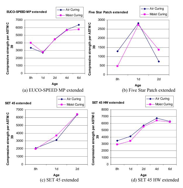
Fig. 3 Compressive Strength Development of Extended Grouts
