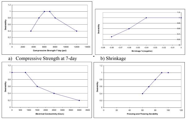
c) Chloride Penetration d) Freezing-and-Thawing Durability Fig. 12 Desirability Function for a) Compressive Strength at 7-day, b) Shrinkage, c) Chloride Penetration and d) Freezing-and-Thawing Durability
