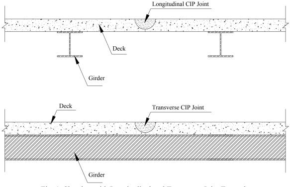
Fig. 1 Sketches with Longitudinal and Transverse Joint Examples
