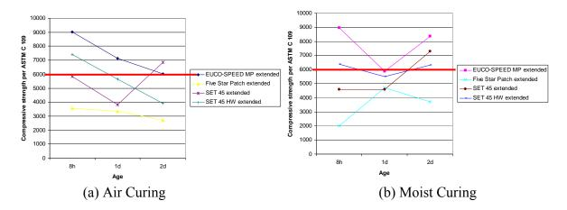
Fig. 6 Compressive Strength Development of the Extended Grouts Per ASTM C109
