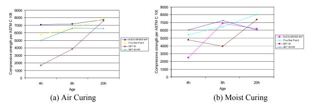
Fig. 10 Compressive Strength Development of the Neat Grouts
