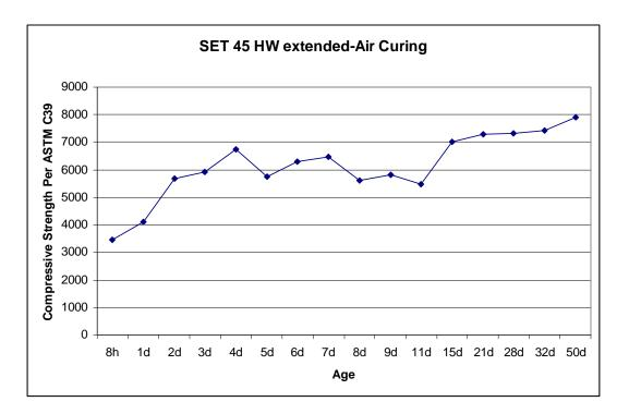
Fig. 7 Compressive Strength Development of SET 45 HW extended Per ASTM C39 (Air Curing)
