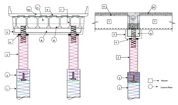
Fig. 9. Precast Seismic Resistant Bridge – Elevation (Left) – Section (Right)
