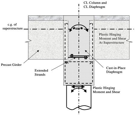
Fig. 3 Typical monolithic moment resistant
