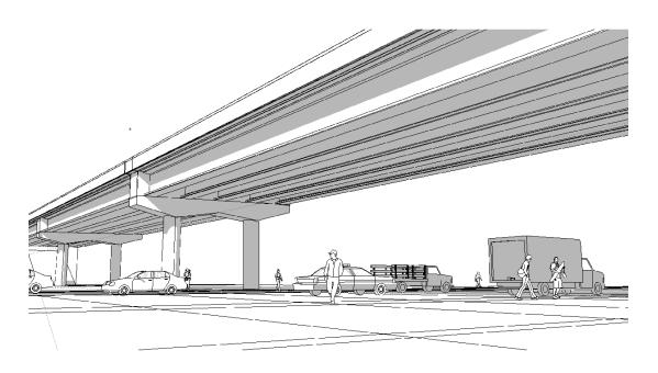
Fig. 7. Computer Rendering of Precast Crossbeam
