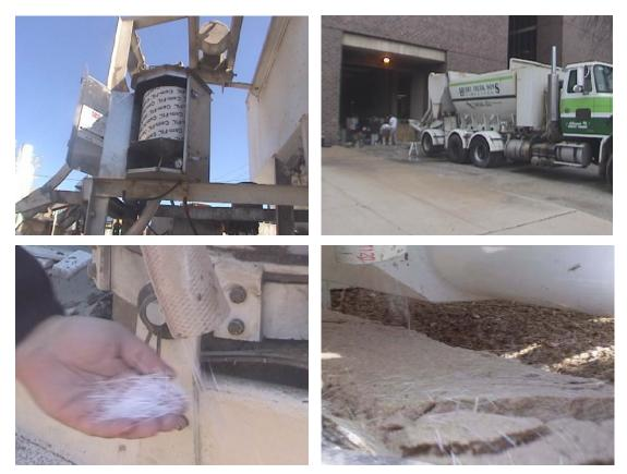
Fig. 2 The new fiber feeder system<sup>4</sup>
