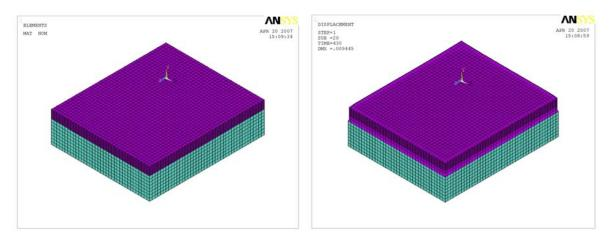
Fig. 6 Meshing of the overlay and slab in the FEA models and typical deformed shape
