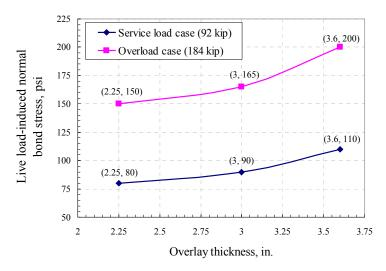
Fig. 4 Overlay thickness versus the live load-induced normal bond stress
