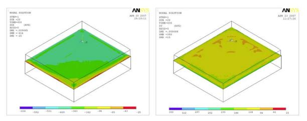
Fig. 7 Typical shear (left) and normal (right) bond stress contours ( $t_o/t_s=0.281$ ,  $E_o/E_s=1$ )
