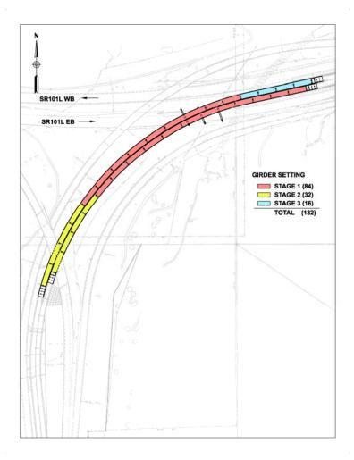
Figure 13 – 132 Girders set in three mobilizations.
