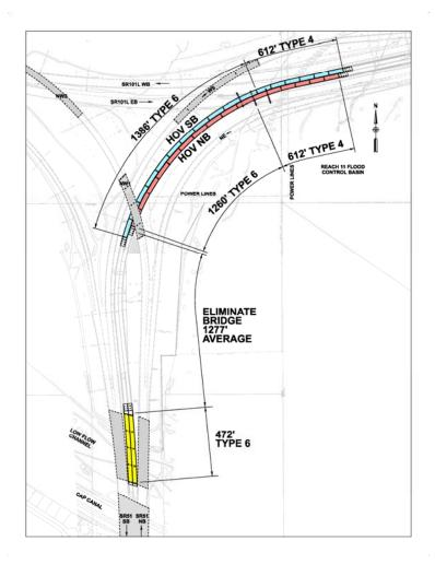
Figure 04 – Cost savings estimated at \$5.5-million was achieved by eliminating over 80,000 square feet of bridge.
