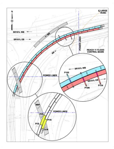
**Figure 09** – Of the many constraints, perhaps the top two are (1) passage under existing Ramp NW bridge with no substructure underneath; and (2) passage over SR101L EB with three cleverly designed straddle bents.
