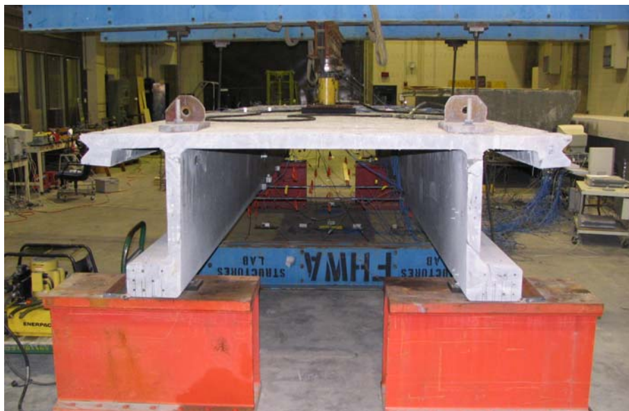
Figure 11. Transverse deck test of first generation Pi girder at Turner Fairbank Laboratory (Photo courtesy of FHWA)
